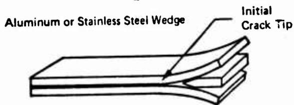
Wedged Crack Extension Specimen - The End and Sides of the Wedge Shall be Approximately Flush with Specimen End and Sides
