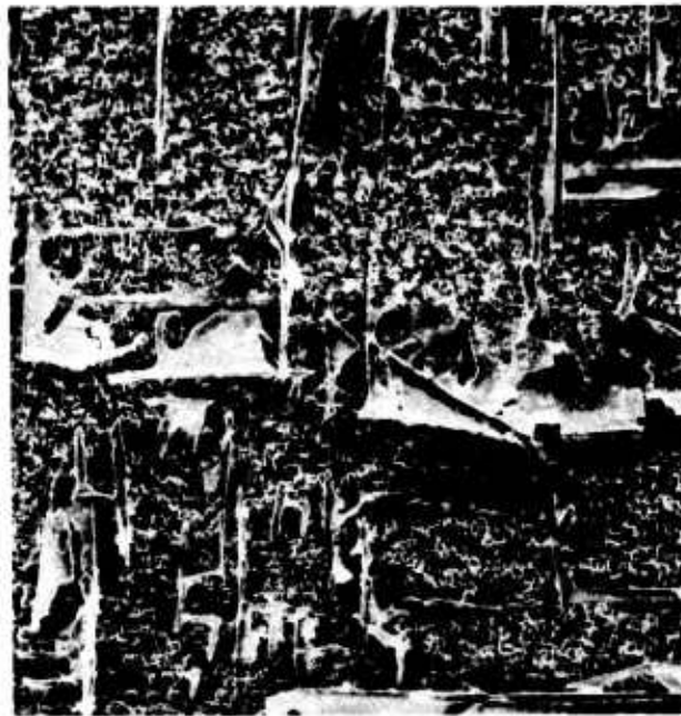
Figure 27. Longitudinal Microstructure of Bar B72 Top Section Illustrating Carbide Dendritic Cells
