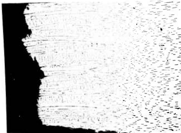
A. 1850°F/30 Ksi 75X FRACTURE IN BAND
