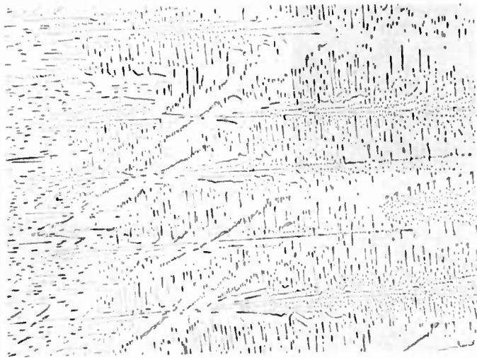
A. Transition From Cells and Dendrites to Aligned Fibers. Light Optical - 100X
