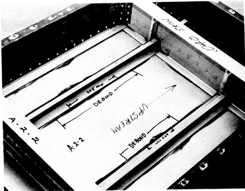
Figure 6. Stiffened Side of Panel A-2-2 (After Acoustic Test)
