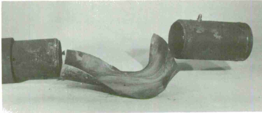
FIGURE 35. Dual-Lined Extended Model Motor Case After Cook-Off Test (RV-7 Propellant)(LHL193542).
