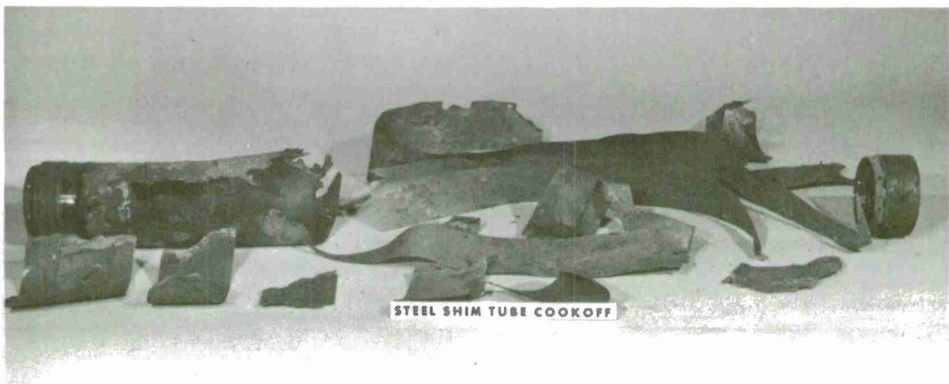
FIGURE 21. Remains of Laminated Steel Spiral Wrapped Tube Cook-Off Test No. 1 (LHL 192362).
