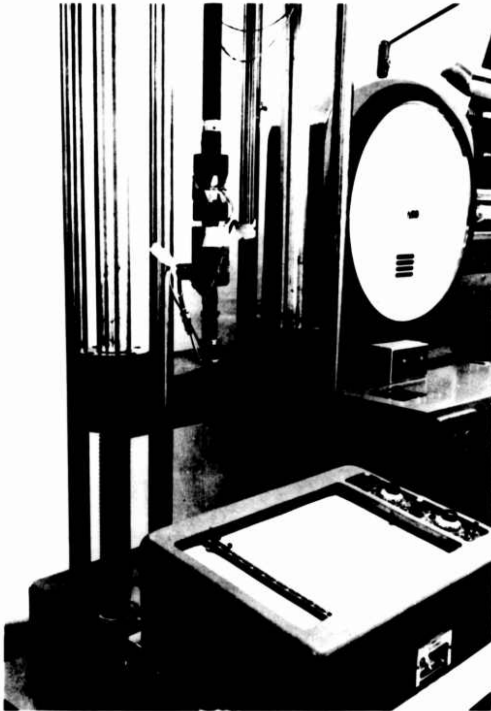
Figure 37 Set-up for Testing Compact Tension Fracture Toughness Specimens
