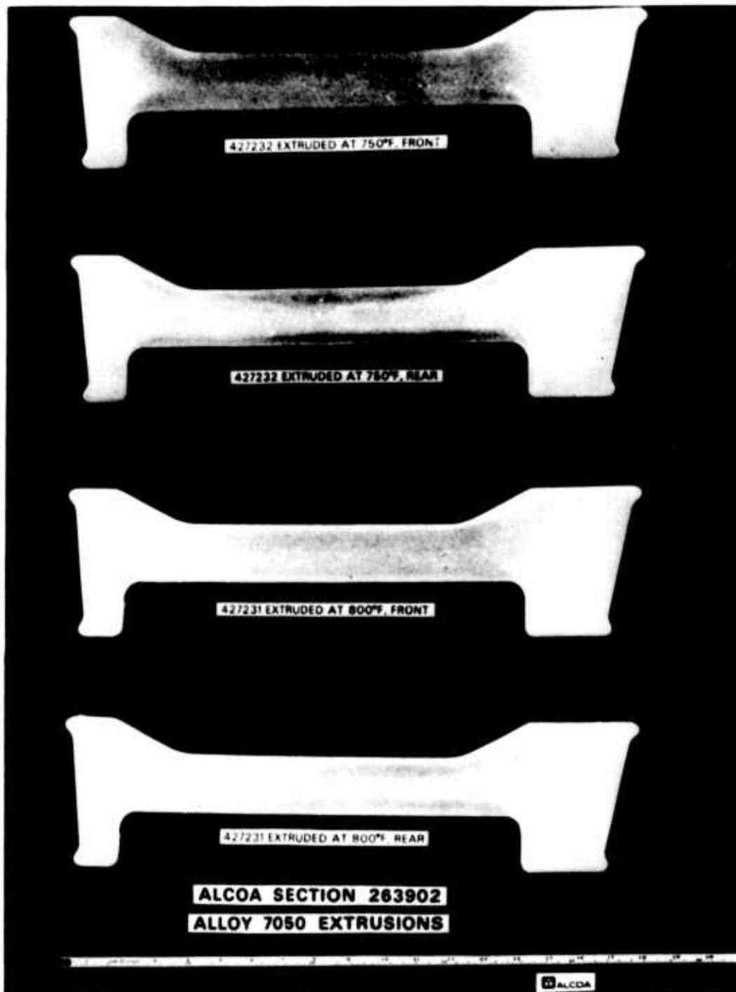
Figure 6 Shows No Significant Effect of Extrusion Temperature on Macrostructure
