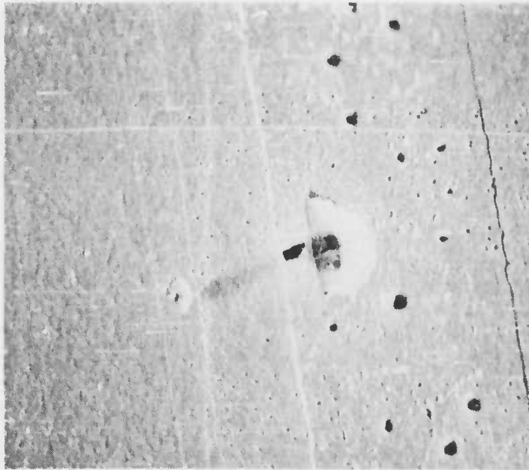
Figure 59. SEM photograph showing subsurface defect where gate-to-source short-circuit occurred.
