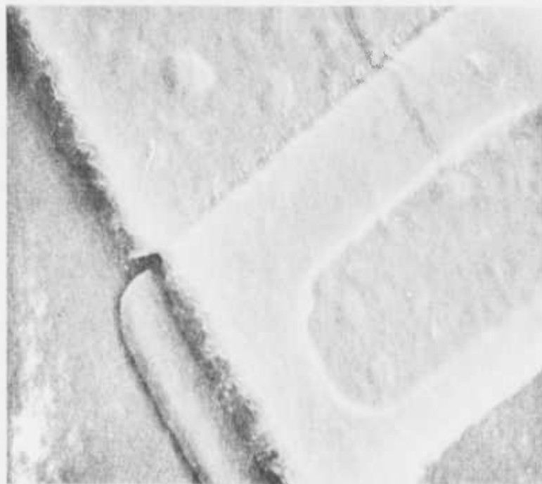
Figure 28. Si-gate TC1092 (#113) after temperature cycling with intermittent bias (3000X).
