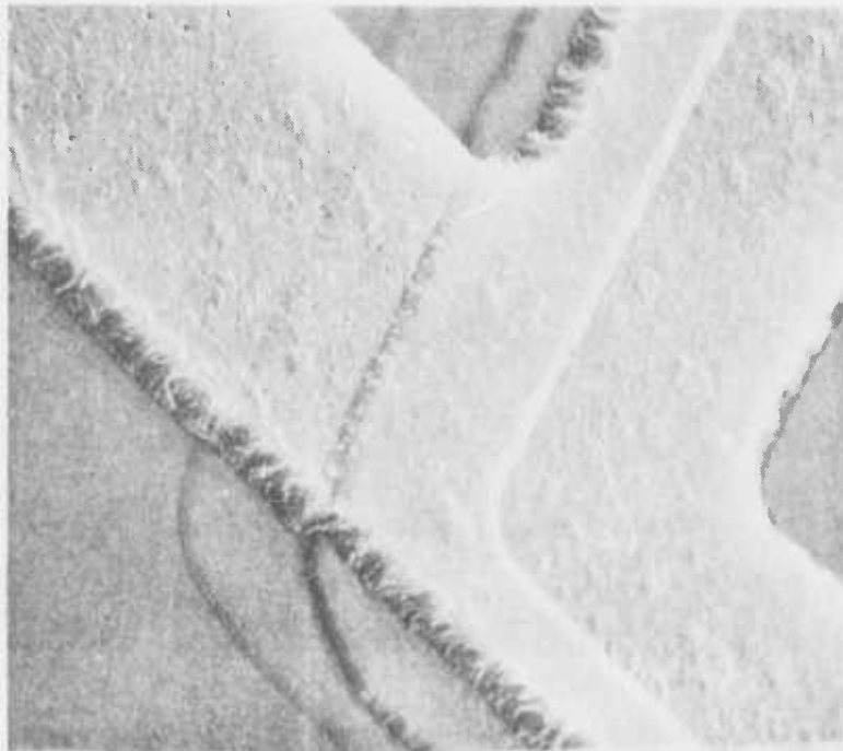
Figure 26. Si-gate TCS056 (#85) after temperature cycling with intermittent bias stress test (3000X).
