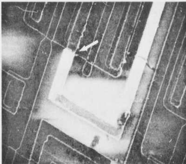
Figure 54. SEM voltage contrast mode (TC1092, #51). Pin 1 - drain terminal, open at epi-island edge.
