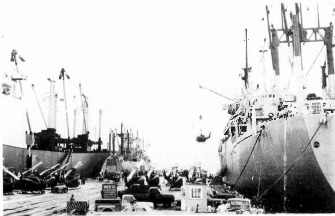
Figure 8-43. Pier 12 was Sufficiently Wide to Provide for the Simultaneous Loading of Three REFORGER Vessels.
