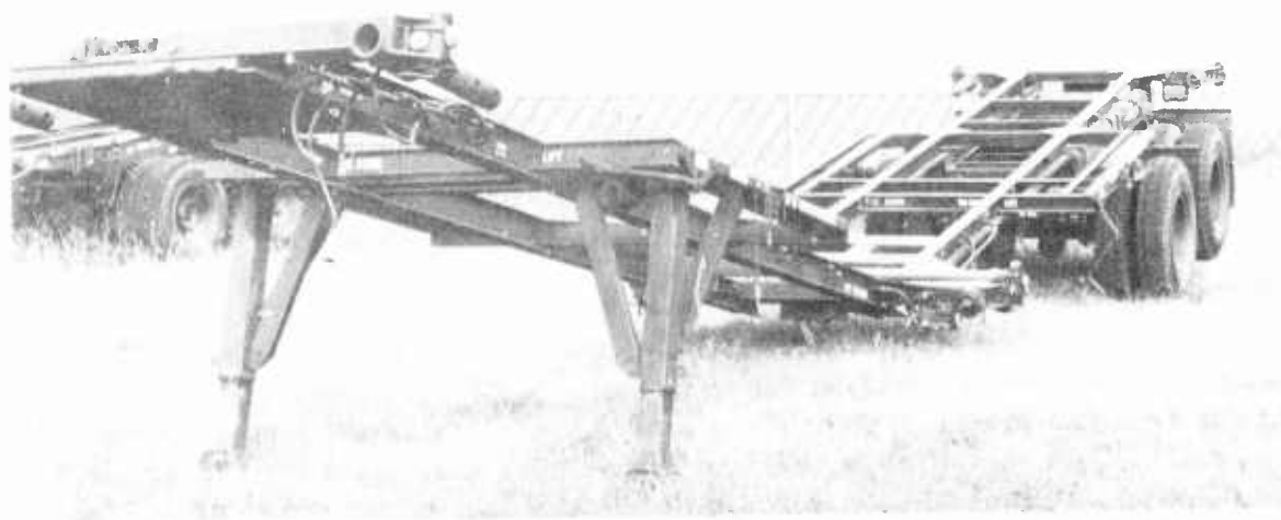
Figure 8-56. MILVAN Chassis Damaged Due to Failure to Install Landing Legs.
