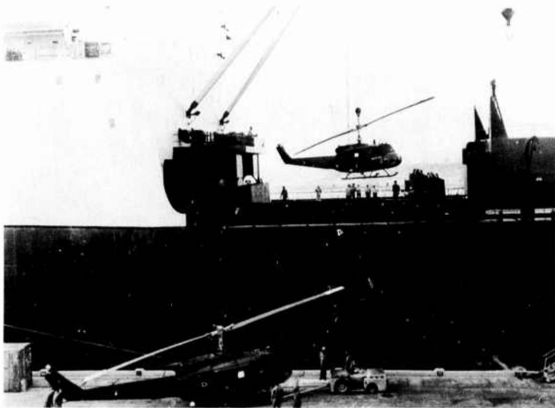
Figure 4-10. Helicopter Positioned for Lowering Through the Hatch.
