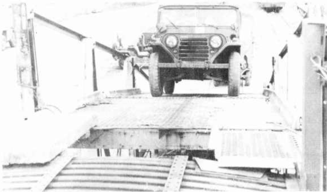
Figure 9-2. Mobile Ramp Used to Load the Bilevel Railcars.
