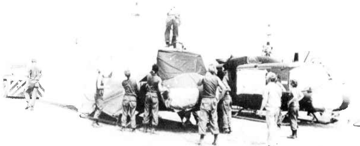
Figure 8-33. Installing Redi-Covers on the UH-1.
