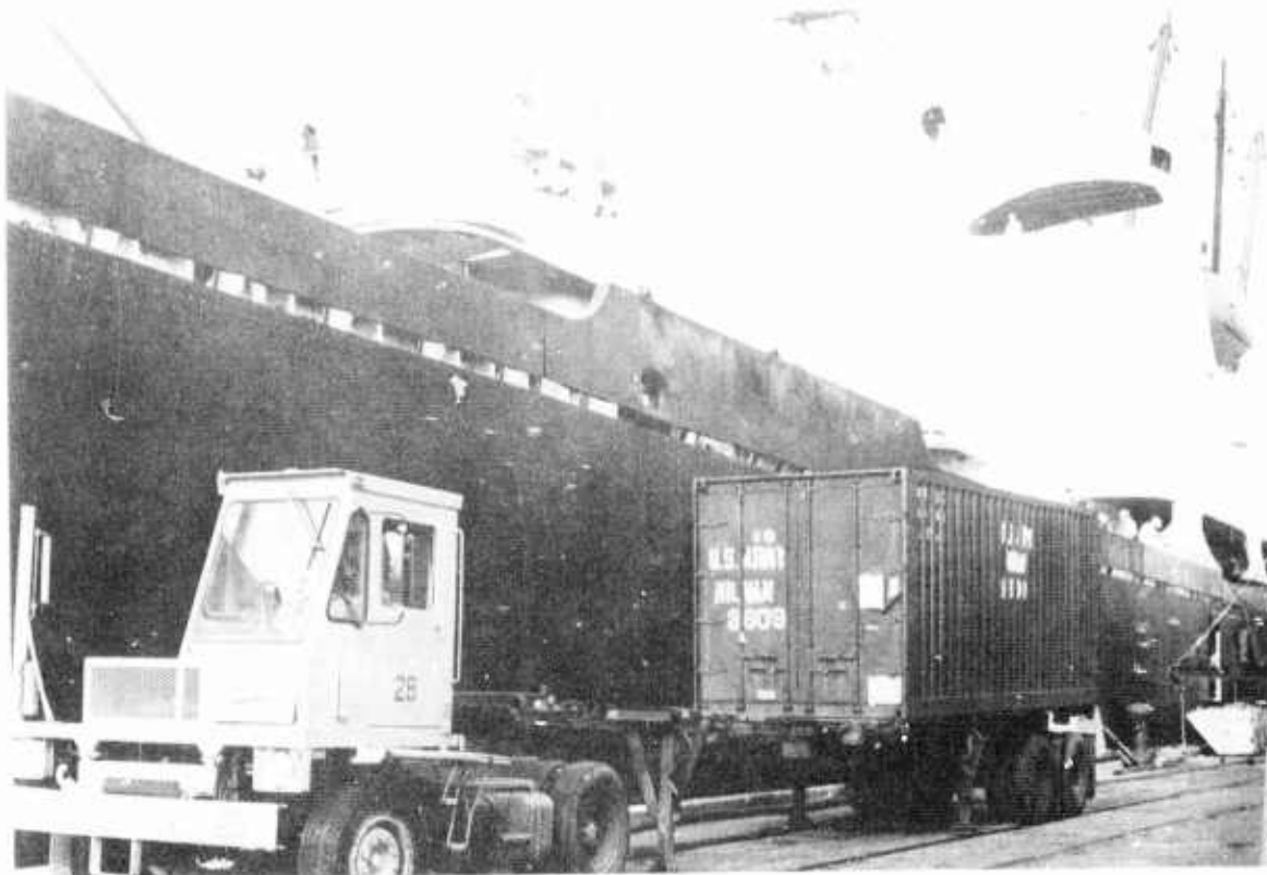
Figure 8-55. To Preclude Damage to the MILVAN Chassis, the Landing Legs on the Second Chassis Must be Installed Prior to Lifting the MILVANS.
