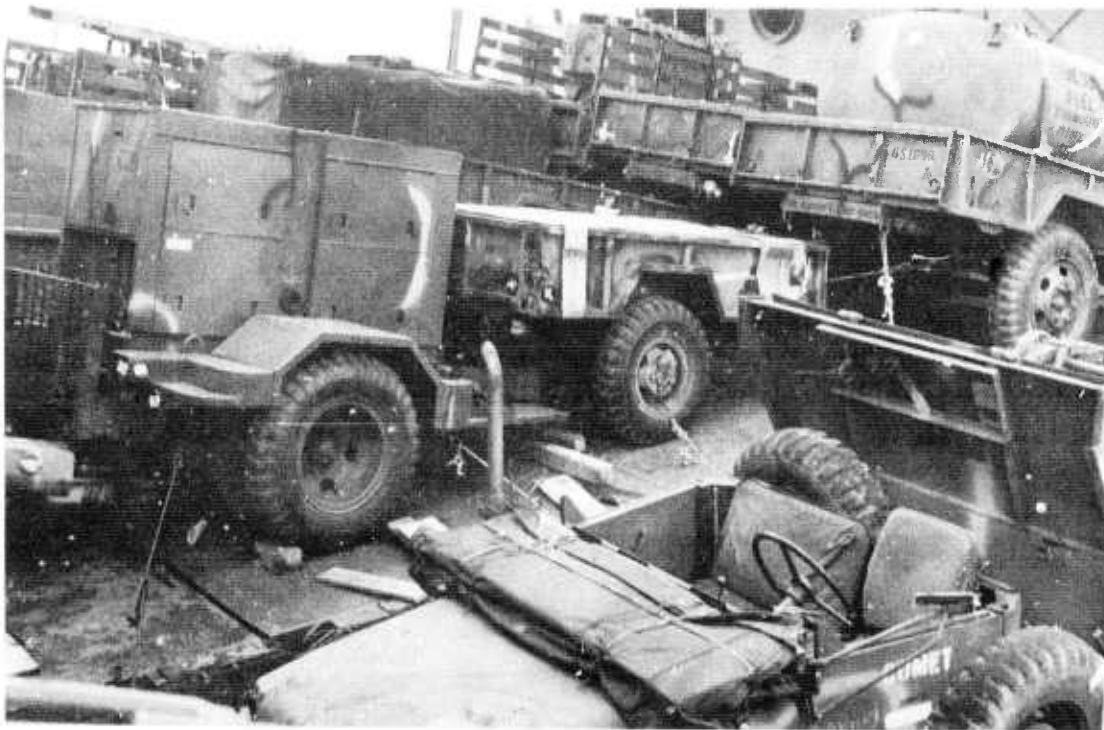
Figure 8-38. Typical Tight Stow of Trailers on Comet .
