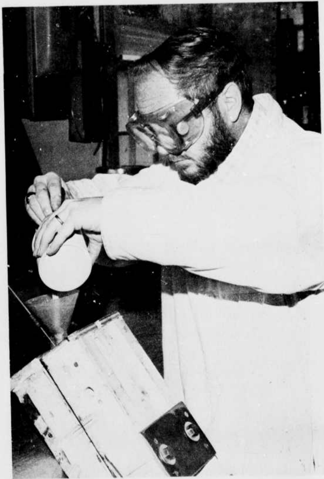
Figure VII-3. Foam Mixture Being Poured into Mold
