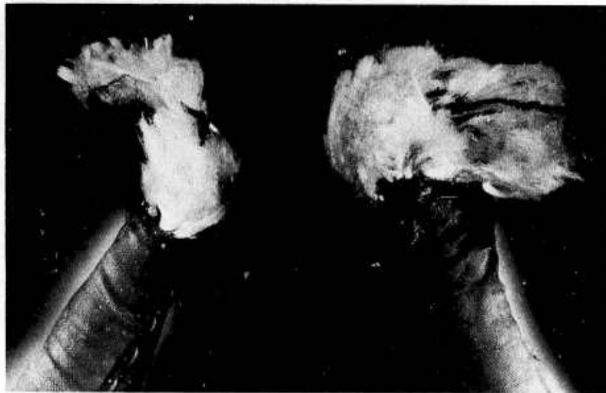
Figure 73. Ruptured Ends of 12000 lb, GR-14 Loadline after Impact with a 1/2 Inch Wide Blunt Missile Nose (actual size)
