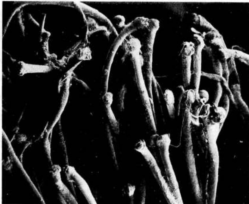
Figure 75. SEM Photograph of Ruptured Fiber Ends from a 12000 lb, GR-14 Loadline that was Impacted at 500 fps by a 1/16 inch Stainless Steel Edge
