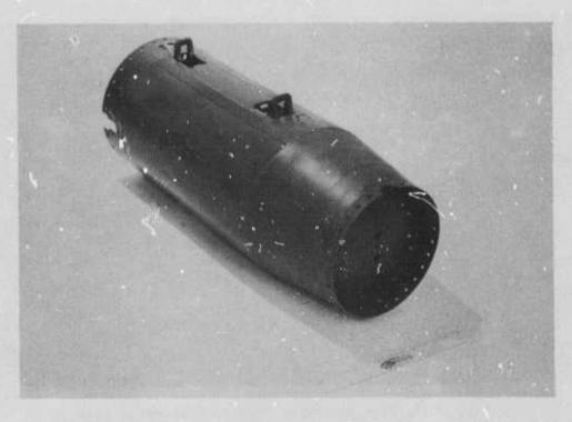
FIG. 3-3. Fuel Tank Assembly Showing Forward Closure.
