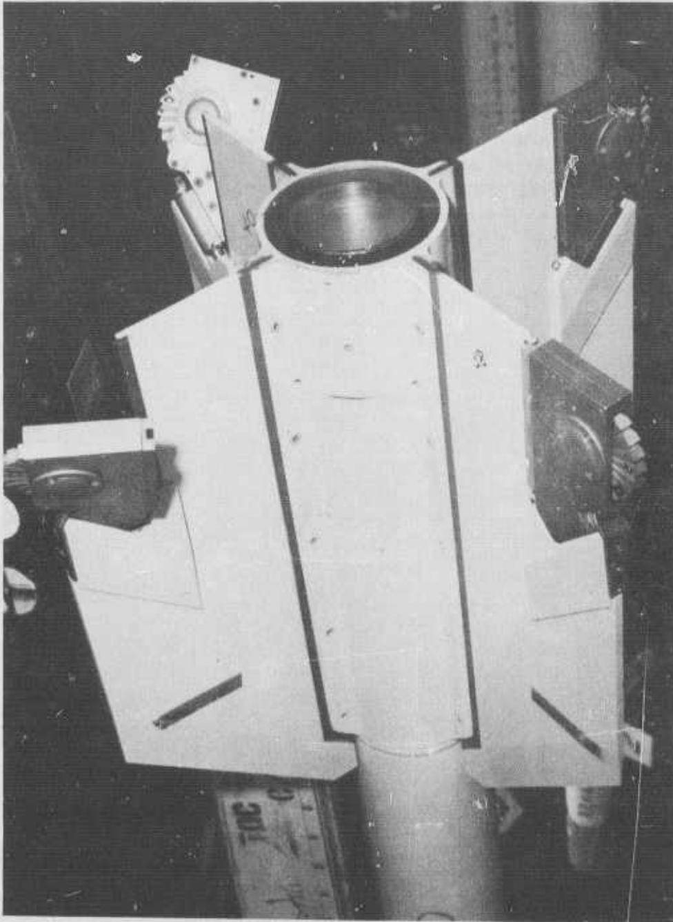
Figure 6. AIM-9J rollerons uncaged following third captive compatibility flight
