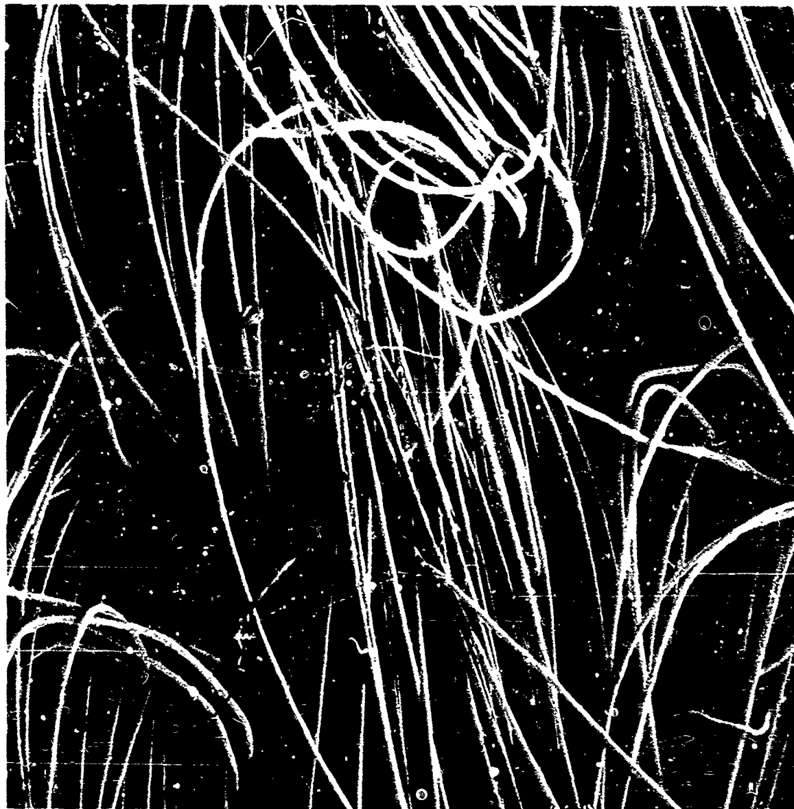
Figure 55. Appearance of Abraded Kevlar Webbing: Unabraded Surface
