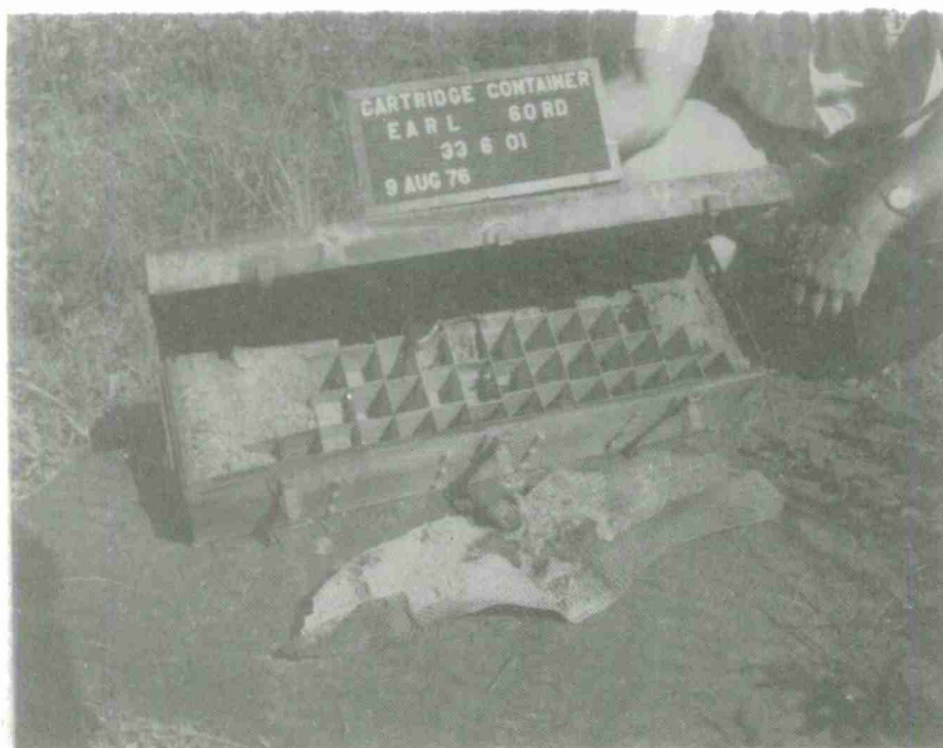
Post External Heat Test "C" Interior View With Venting Cover in Foreground
