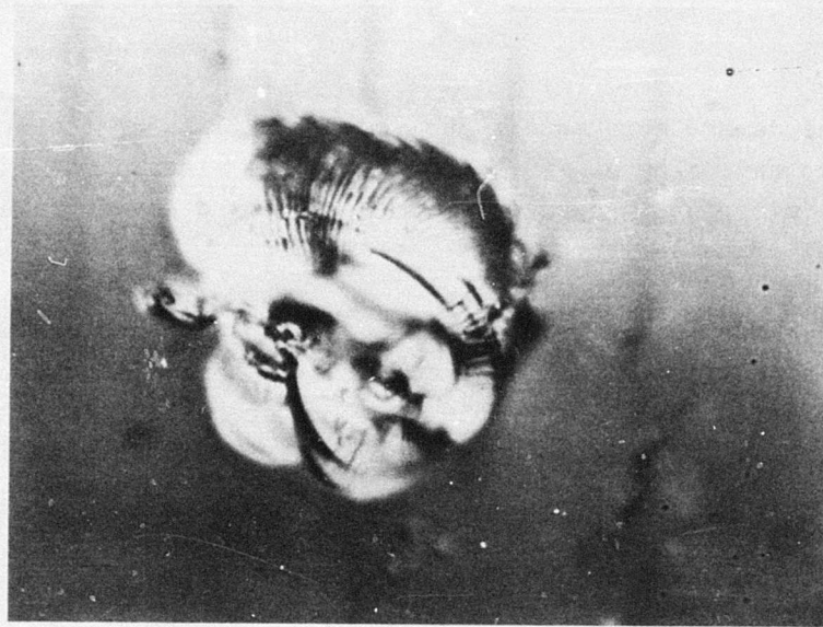
Figure 120. Optical Micrograph in Bright Field Reflected Light of Surface Relief Fracture Formed in Ion Exchanged Glass after 60 sec Exposure to Standard Rainfield (900X)
