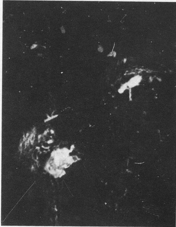
Figure 46. Ductile Nature of Polysulfone in Vicinity of Pits Formed Along Surface Scratches (1000X)
