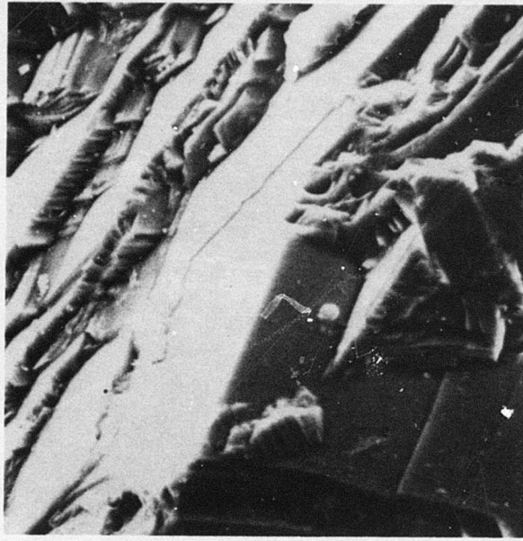
Figure 71. Scanning Electron Micrograph of Bend Bar Fracture of CVD Zinc Selenide (1500X)
