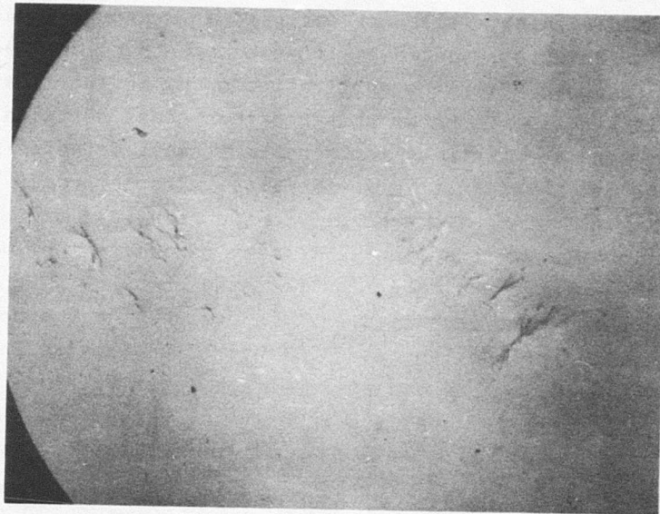
(b) Oblique Reflected Light Micrograph of Initial Crack Arrays (280X)
