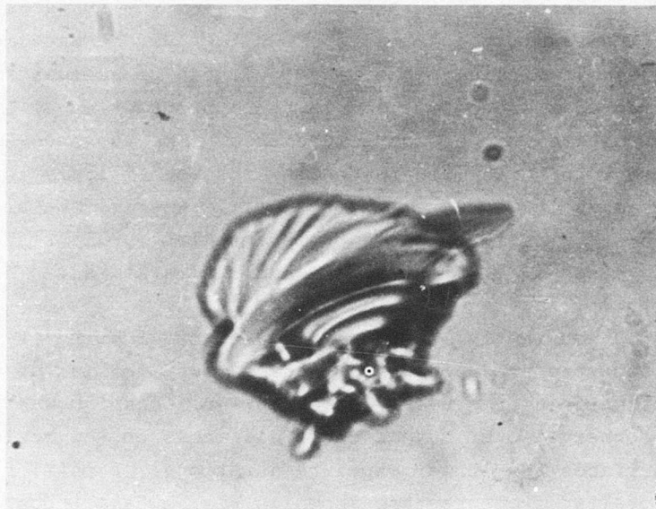
(b) Transmitted Light Micrograph of Median Vent Fracture (400X)
