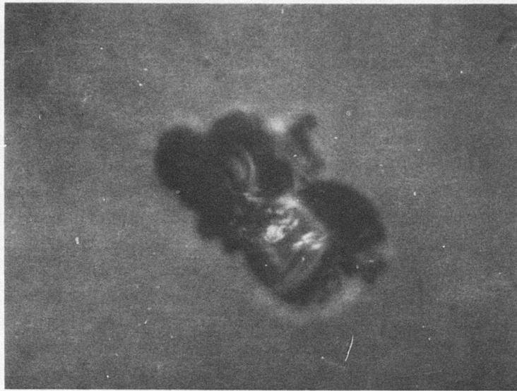
(a) Polarized Reflected Light Micrograph of Subsurface Relief Fracture (600X)
