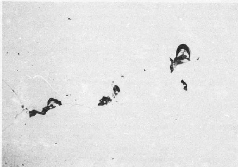
Figure 107. Optical Micrograph in Oblique Reflected Light of Linear Crack Array in Soda Lime Glass after 10 min. Exposure to 1 in/hr Rainfall at 730 fps in AFML Facility (320X)
