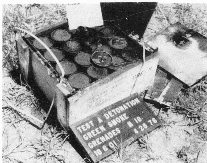
Figure 3. Typical Test Results, Green Smoke Grenades.
