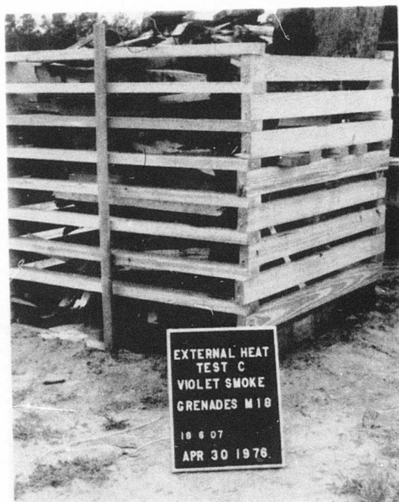
Figure 8. Typical Funeral Pyre for C Tests.
