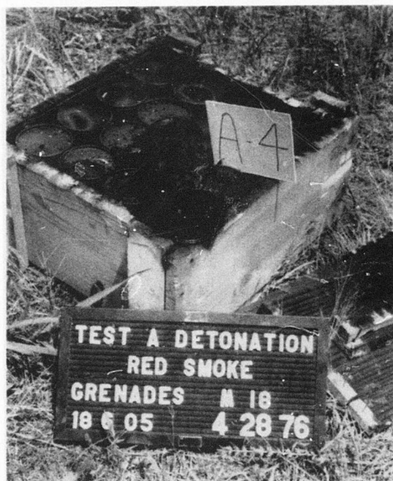
Figure 6. Typical Test Result, Red Smoke Grenades.
