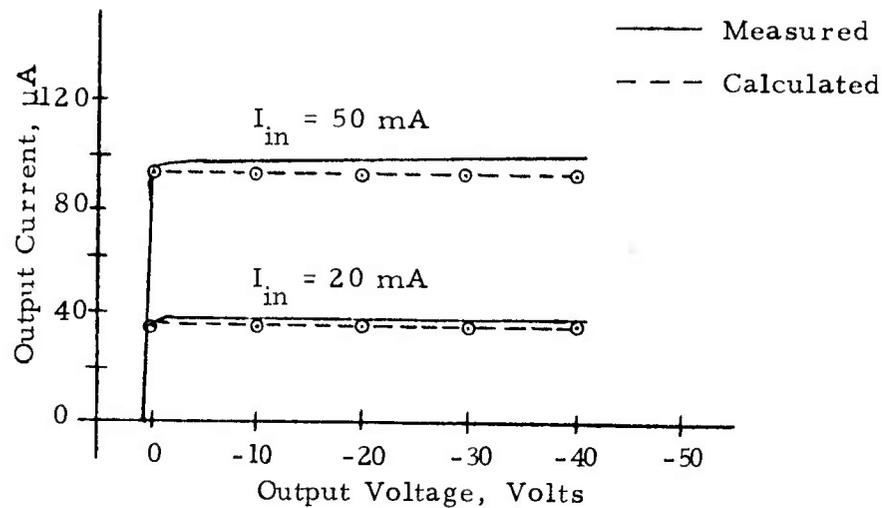
Figure 4-5. MCD2 output current-voltage characteristic.
