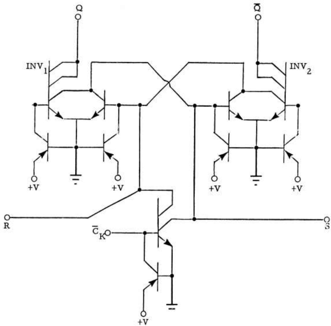
Figure 3-7. I<sup>2</sup>L R-S flip-flop schematic.
