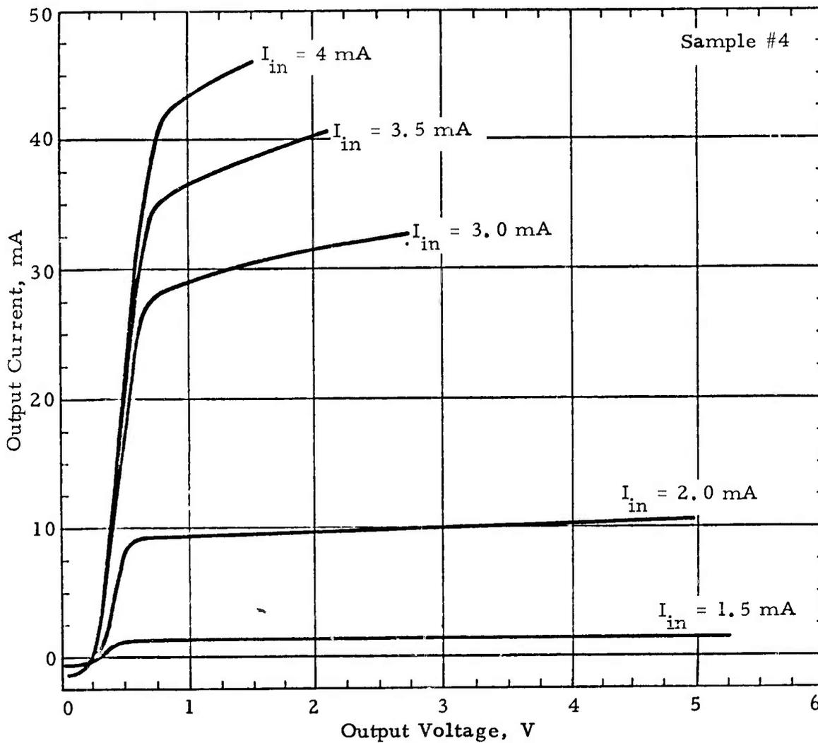
Figure 4-13. HP 4360 output current-voltage characteristics.
