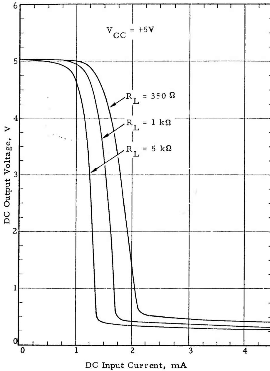
Figure 4-12. HP 4360 diode/gate coupler dc transfer characteristic.
