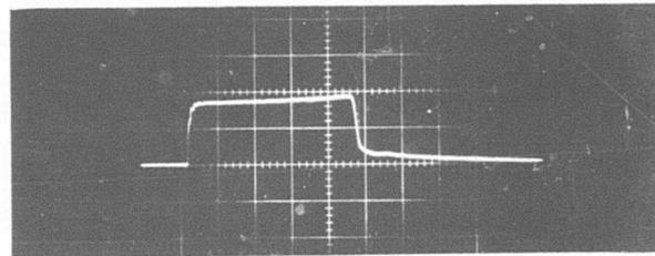
Figure 2-2. CD4023A narrow-pulse photoresponse waveforms, input bias 1-1-1, 0-output state.
