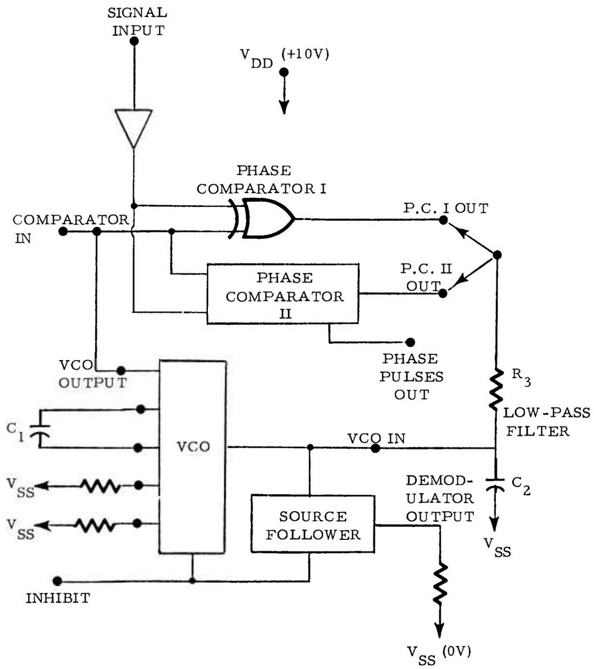
Figure 2-18. CD4046A phase-locked loop schematic.
