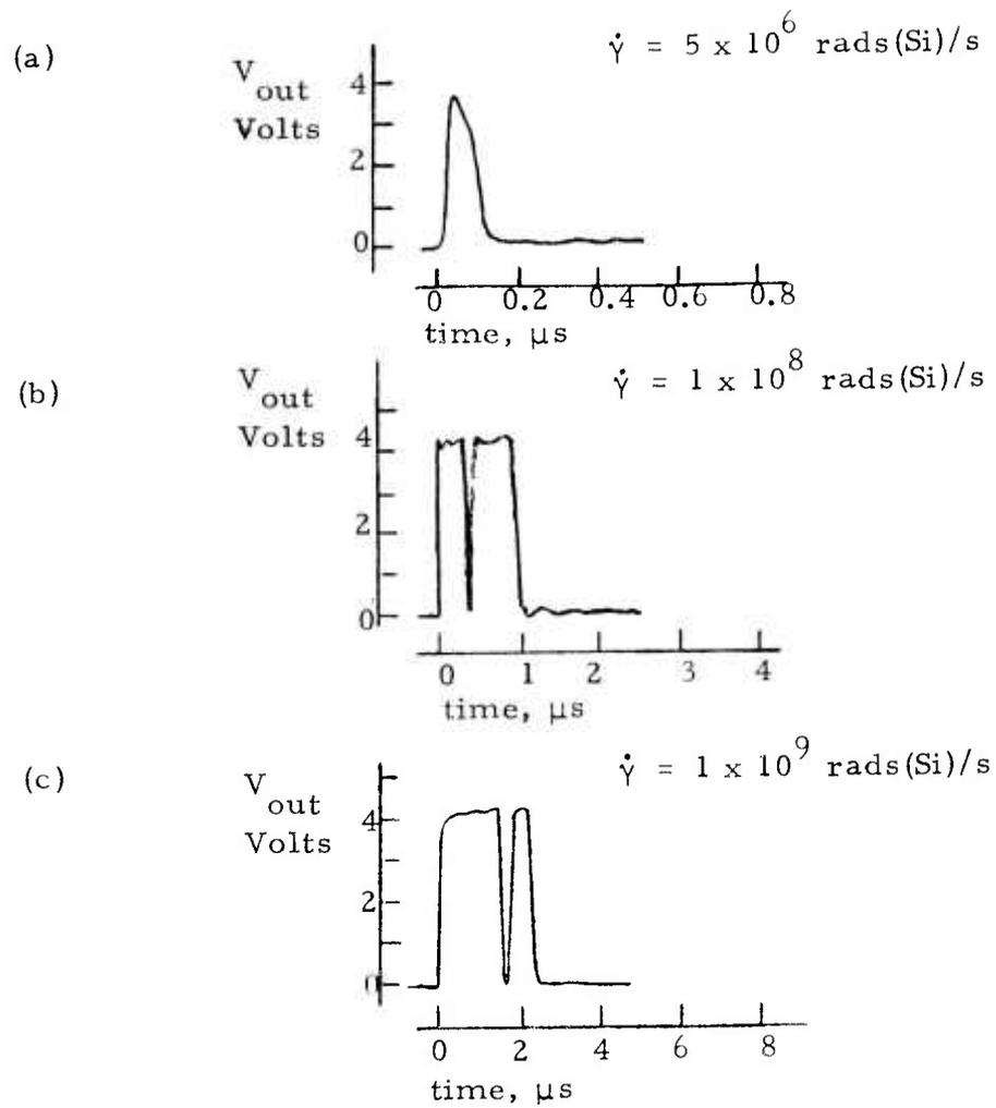
Figure 4-21. HP4364 narrow-pulse photoresponse waveforms,
