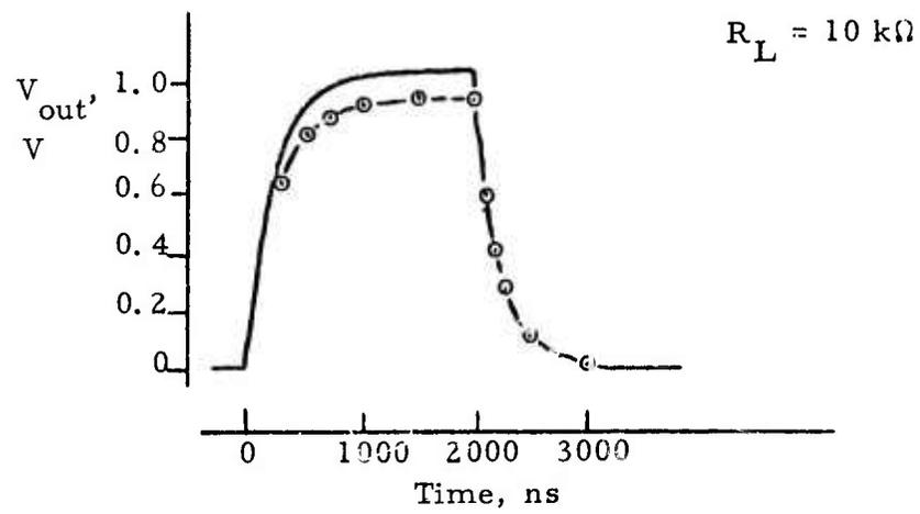
Figure 4-9. MCD2 output switching response, pulsed input current,  $I_{in} = 50 \text{ mA}$ .
