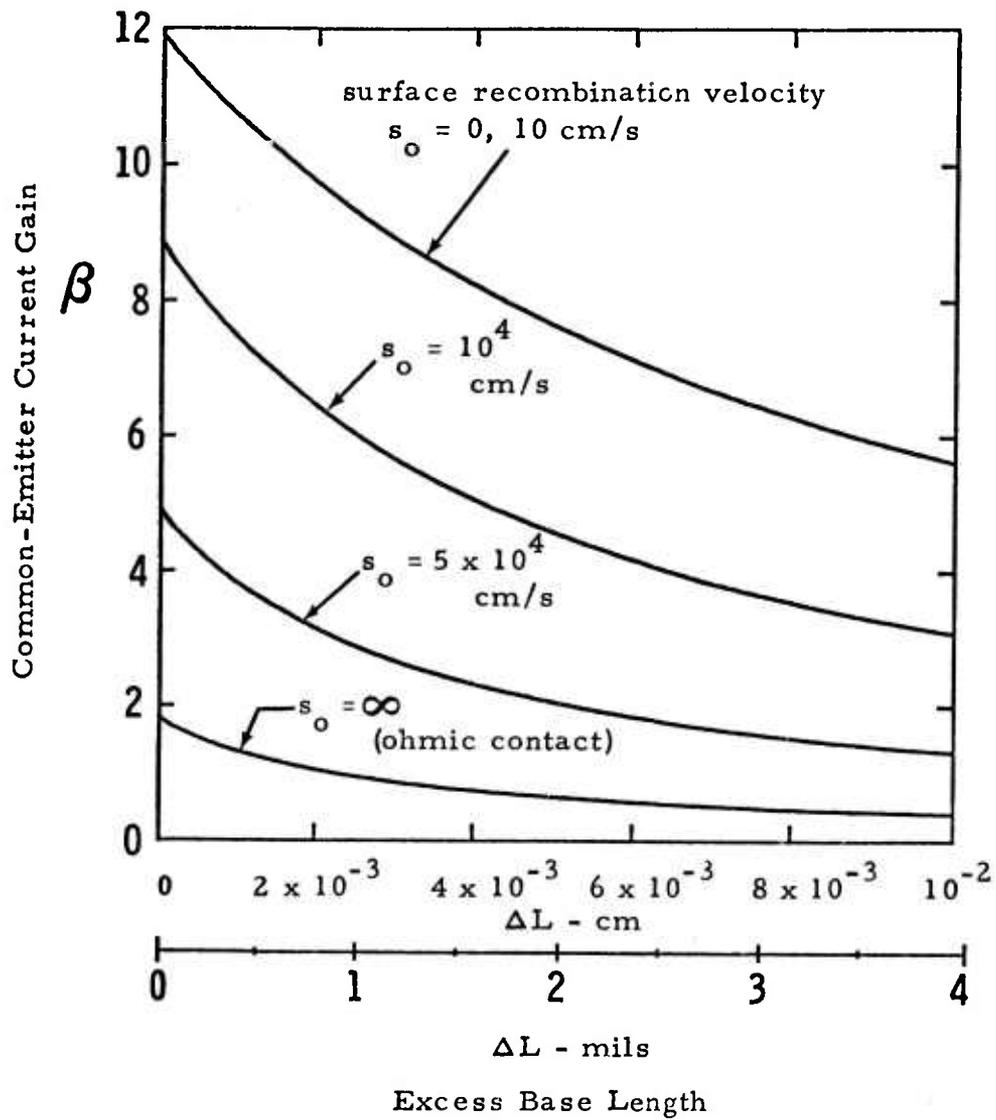
Figure 3-5. Npn transistor-base surface effects.
