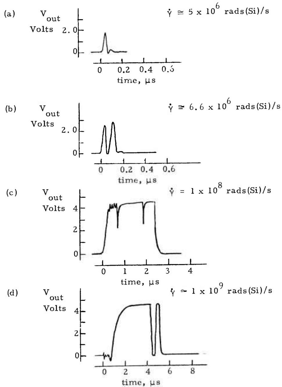
Figure 4-18. HP4360 narrow-pulse photoresponse waveforms,
