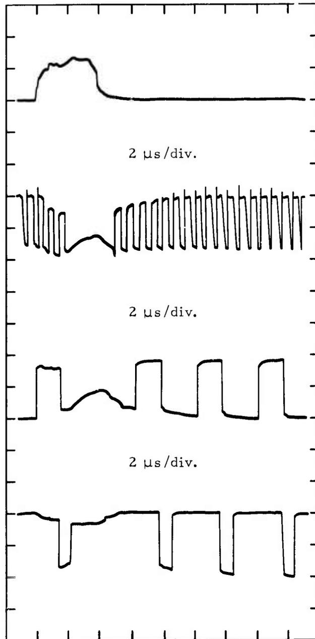
Figure 5. MC1678L ECL Four-bit Counter Wide-Pulse Photoresponse.
