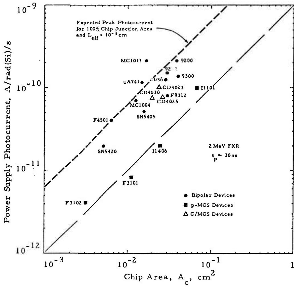
Figure 6. MSI/LSI Array Power Supply Photocurrents.
