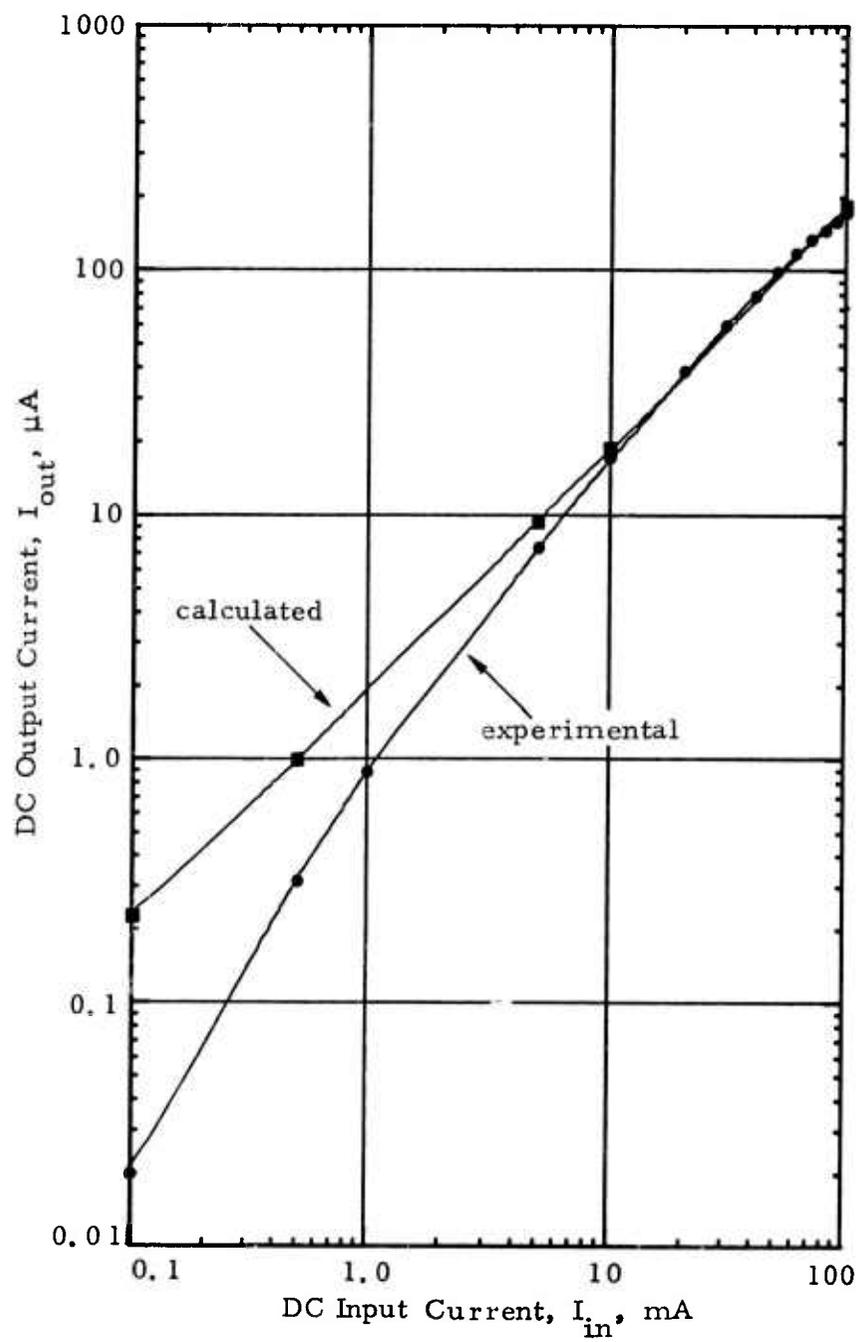
Figure 4-4. Measured and calculated MCD2 current-current transfer characteristics.
