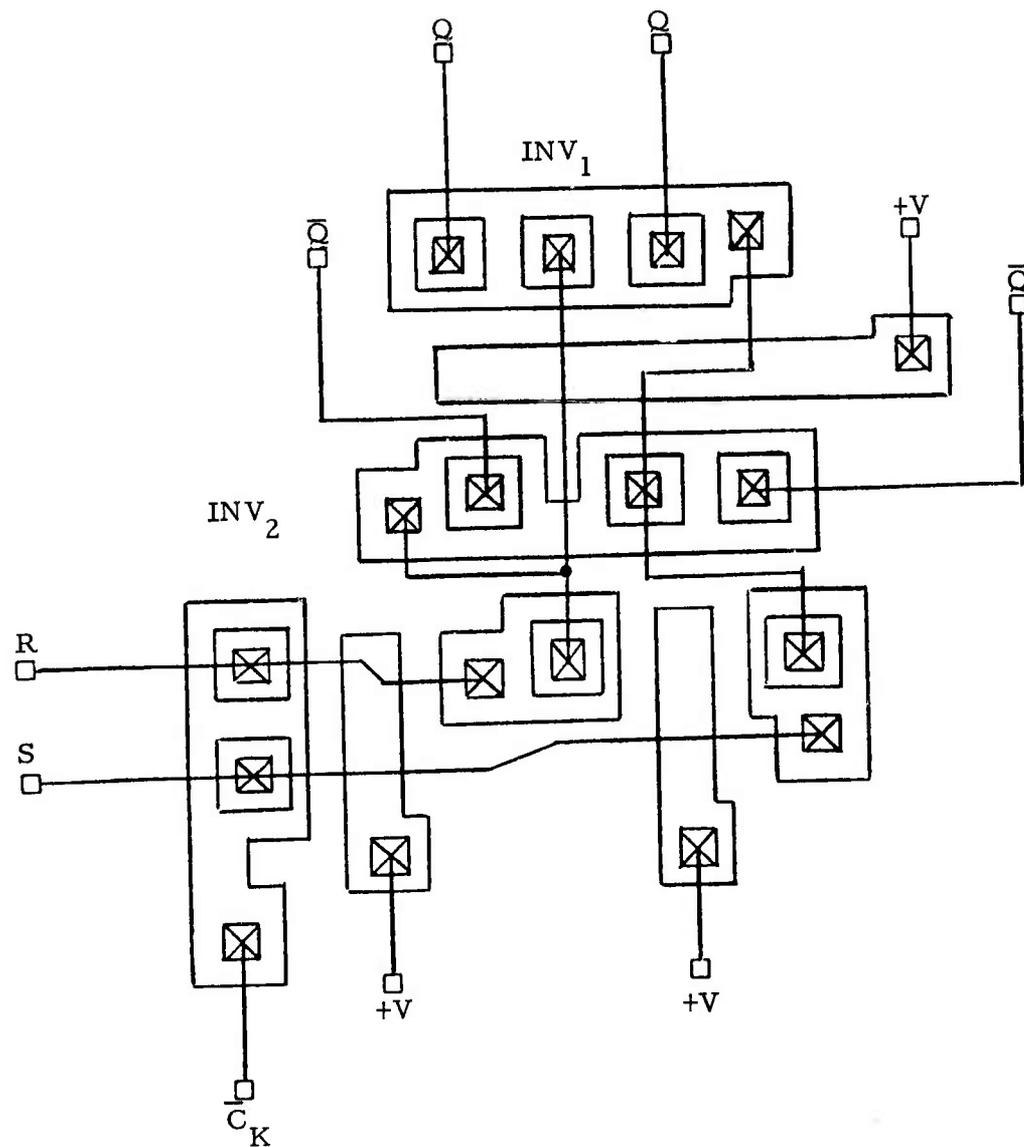
Figure 3-8. Simplified layout of the  $I^2L$  R-S flip-flop.
