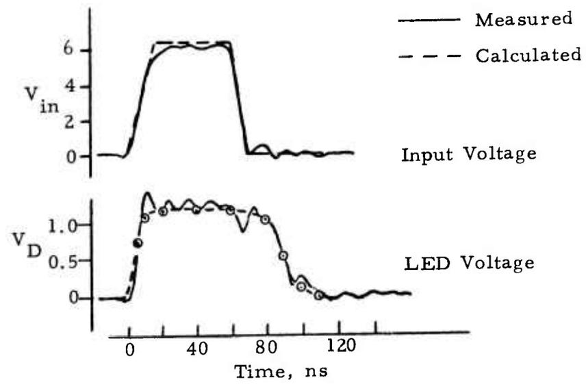
Figure 4-7. MCD2 input switching response.
