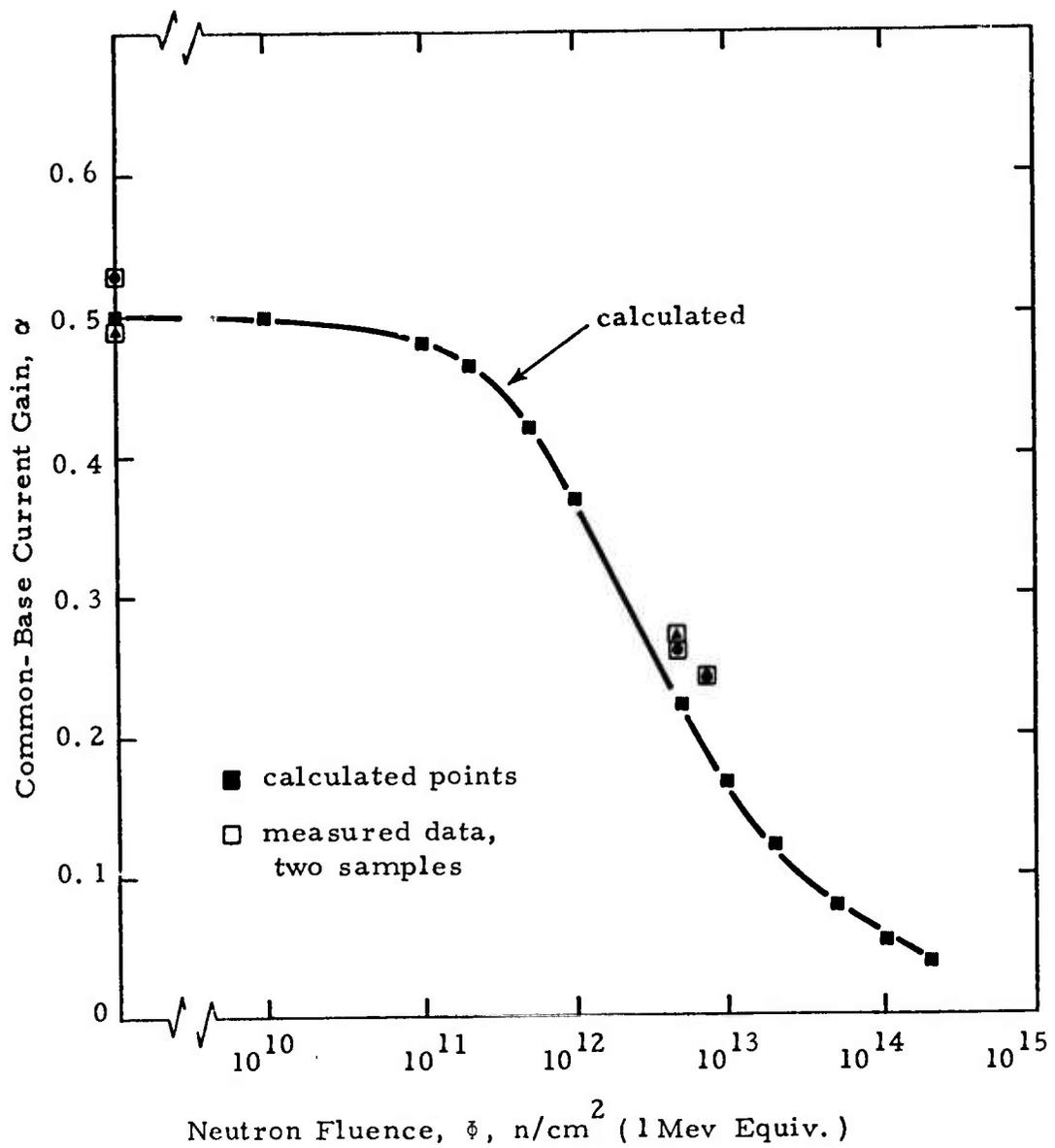
Figure 3-3. 7L pnp transistor element gain degradation.
