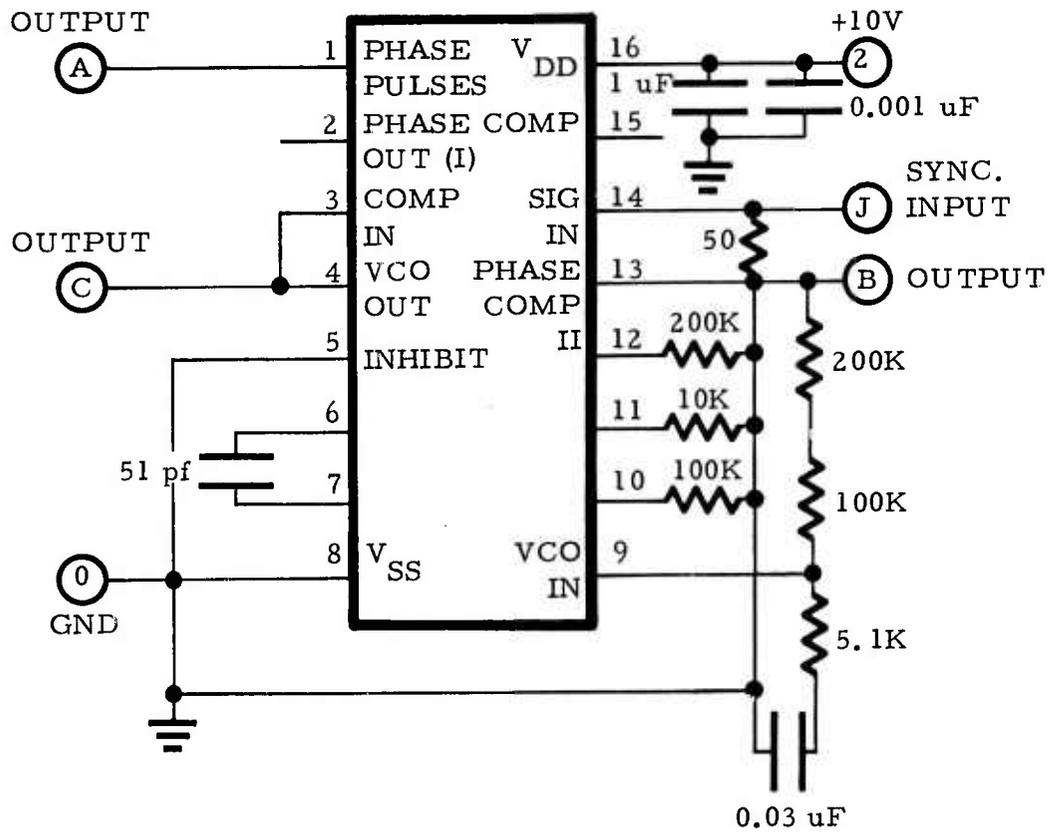
Figure B-10. CD4046A, phase-locked loop, Phase Comparator II, test circuit.
