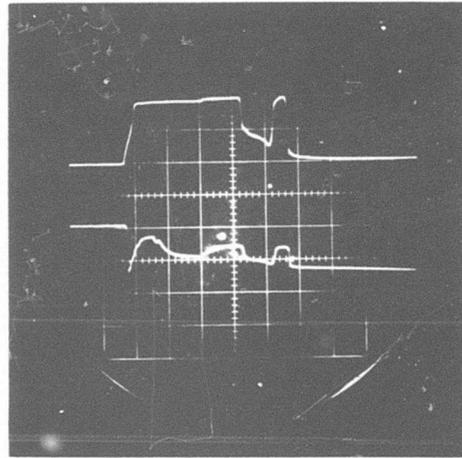
\* Note, both  $Q$  and  $\bar{Q}$  outputs = 0 well after the end of the radiation pulse
