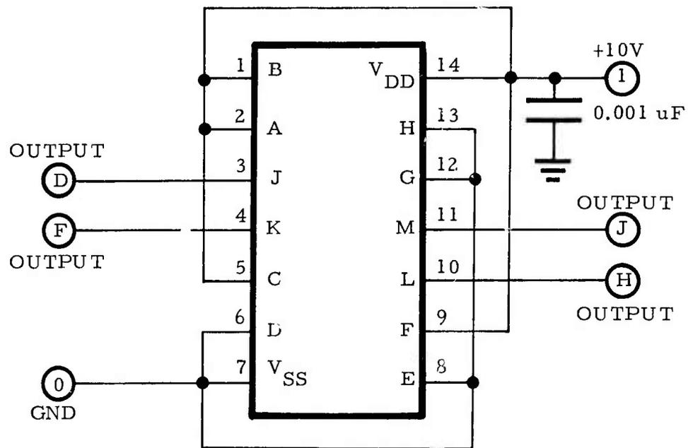
Figure B-5. CD4030A, quad exclusive-OR gate, static input test circuit.
