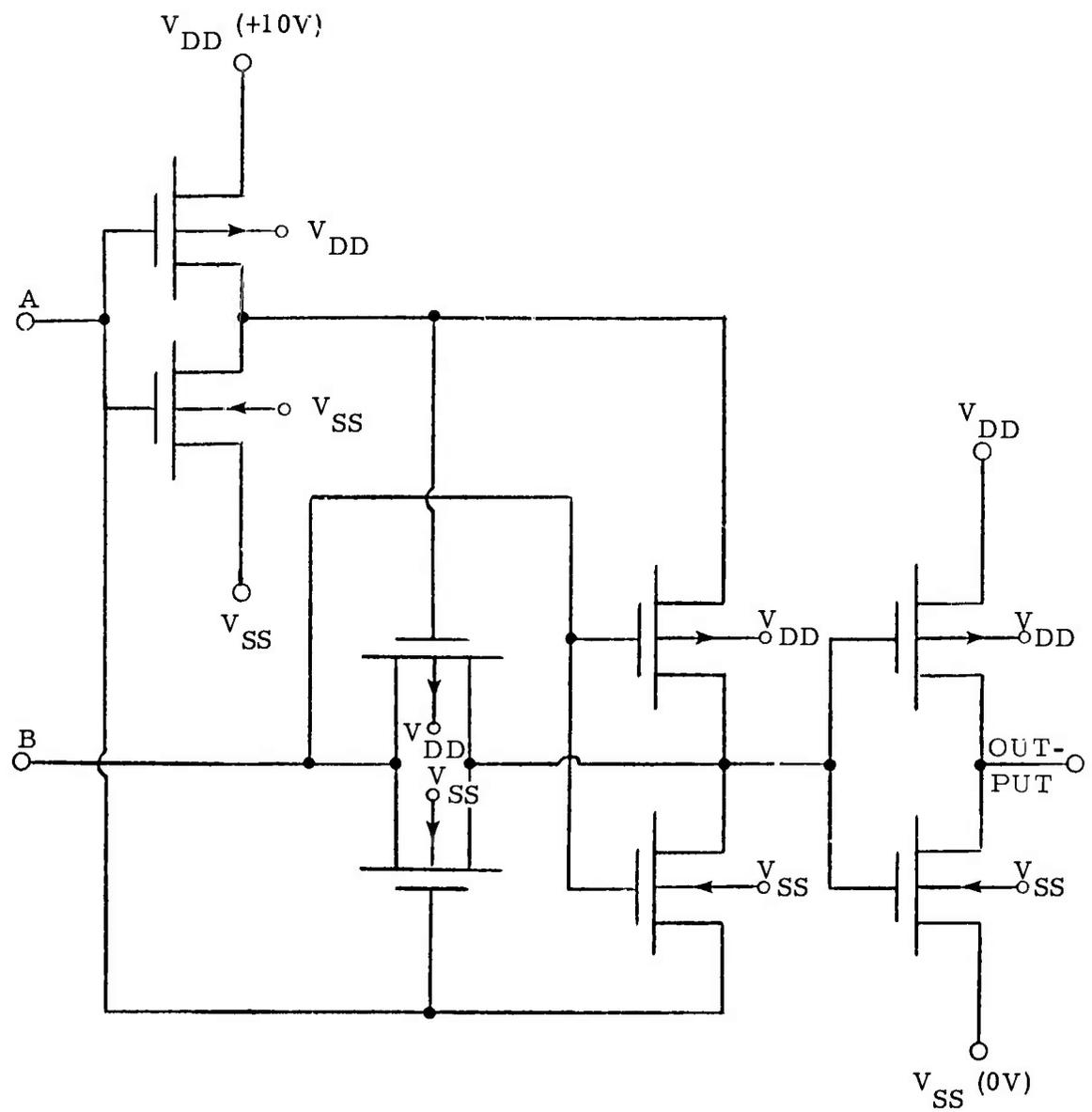
Figure 2-9. CD4030A exclusive-OR gate schematic.
