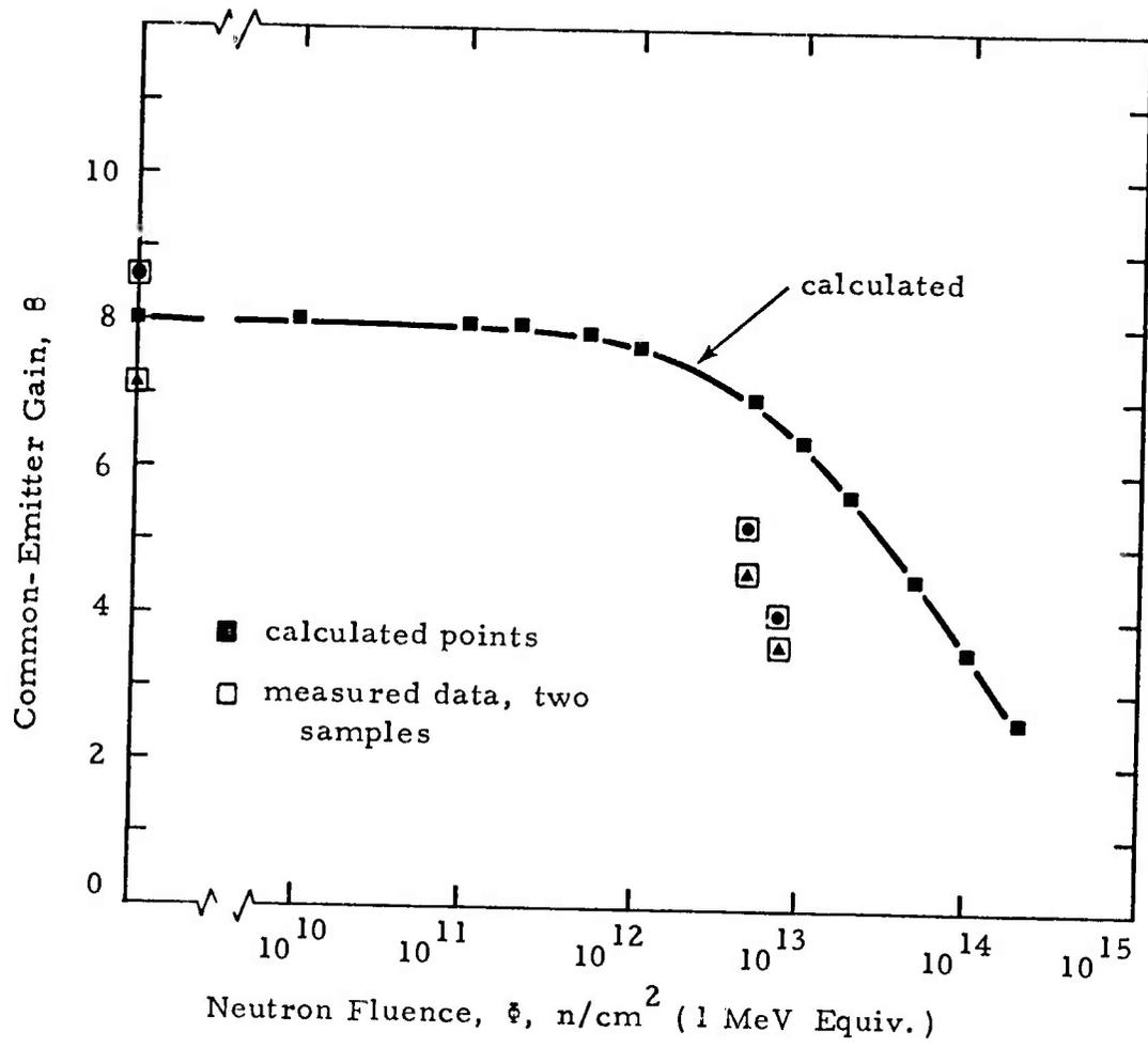
Figure 3-4.  $1^2\text{L}$  npn transistor gain degradation.
