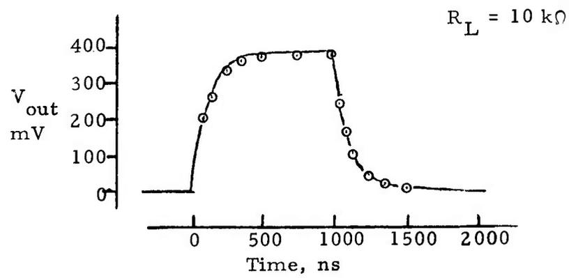
Figure 4-8. MCD2 output switching response, pulsed input current,  $I_{in} = 20\text{ mA}$ .
