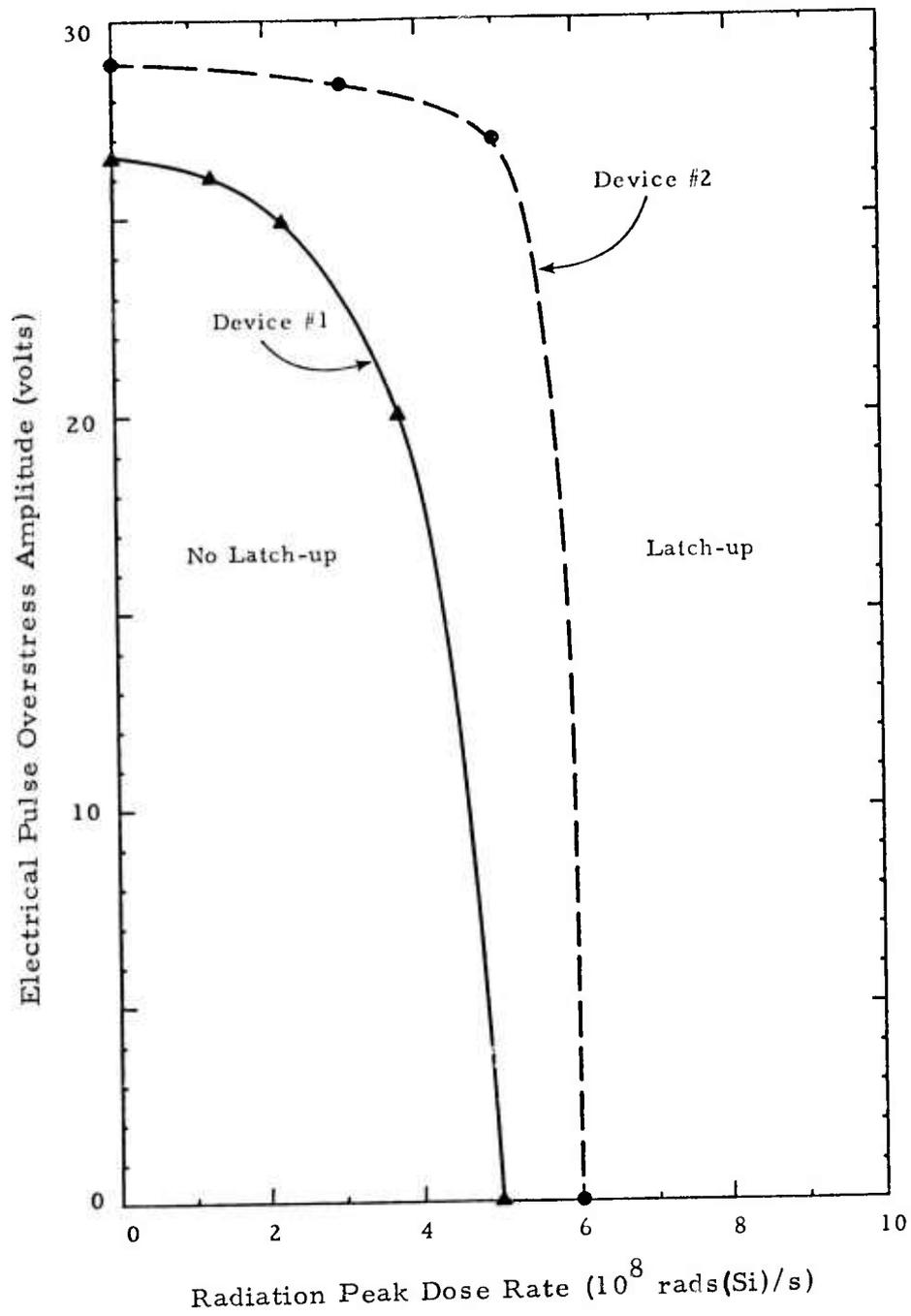
Figure 5-2. Threshold for latch-up in combined EPO-radiation environment.
