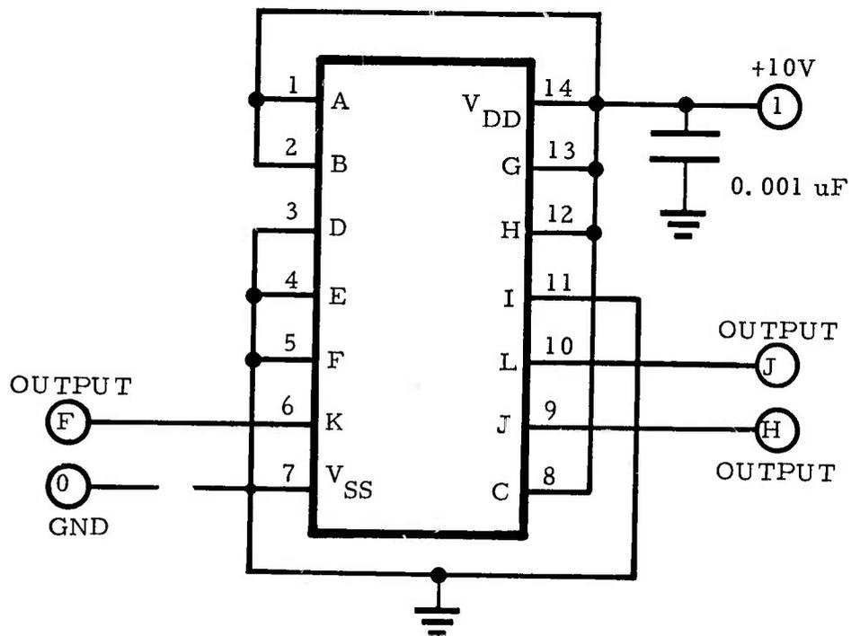
Figure B-1. CD4023A, triple 3-input NAND gate, static input test element.
