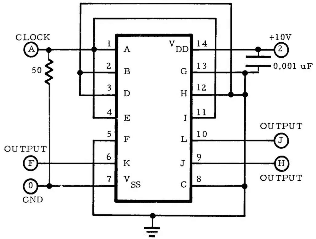
Figure B-4. CD4025A, triple 3-input NOR gate, dynamic input test circuit.
