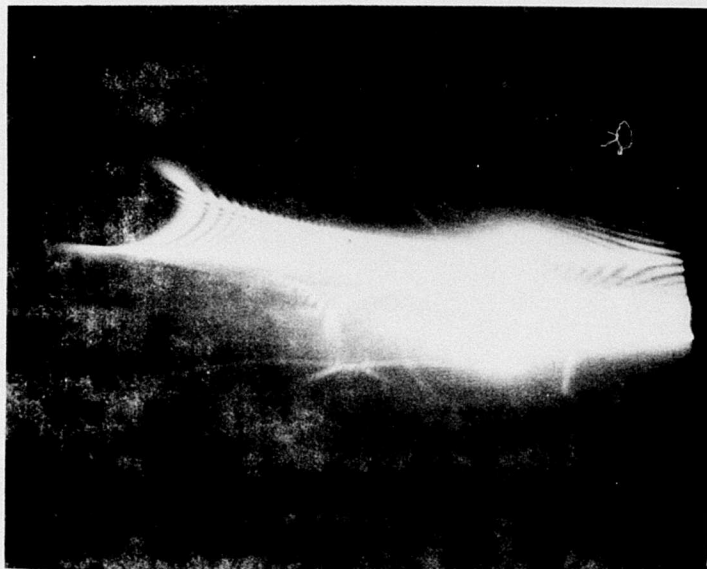
Figure 1. Samples of the Types of Laser Reflections Observed from Ice Imaged on a Card Placed 0.5 to 1.0 m from the Ice Surface.
