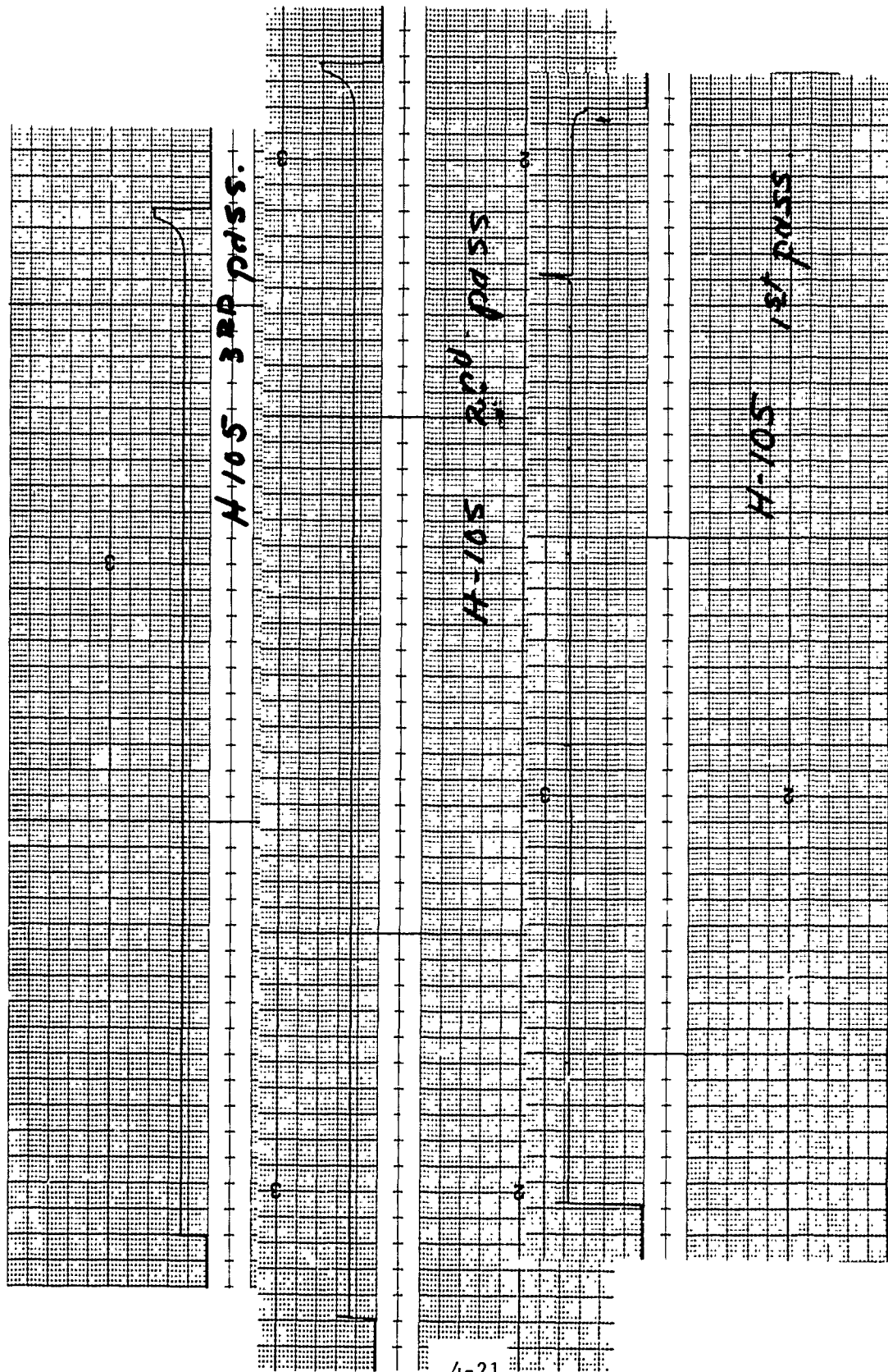
Figure 4.1.5-6 TYPICAL BEAM CURRENT OSCILLOGRAPHIC TRACE
