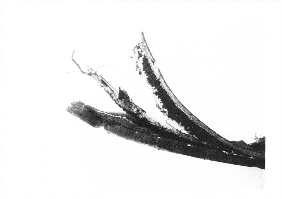
Figure 15. Closeup Photograph of a Cross-Section in a Modified Tread Band After Tensile Failure.
