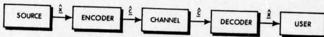
Figure A.1-1 Classical Communication System Configuration
