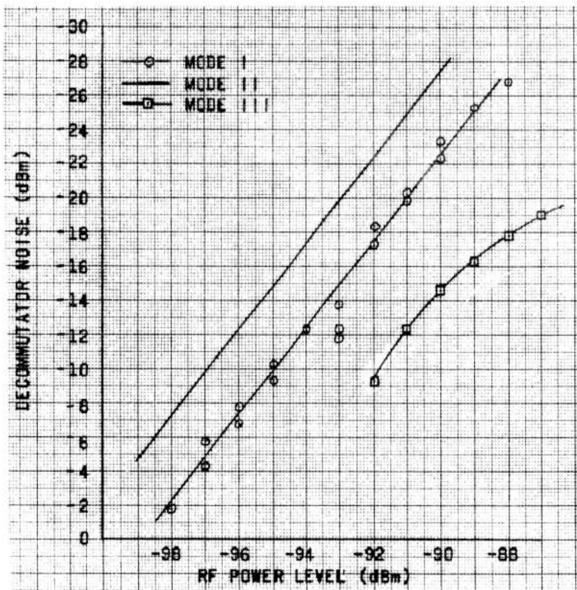
Figure 4. Relation Between Decommulator Noise and RF Power Level.
