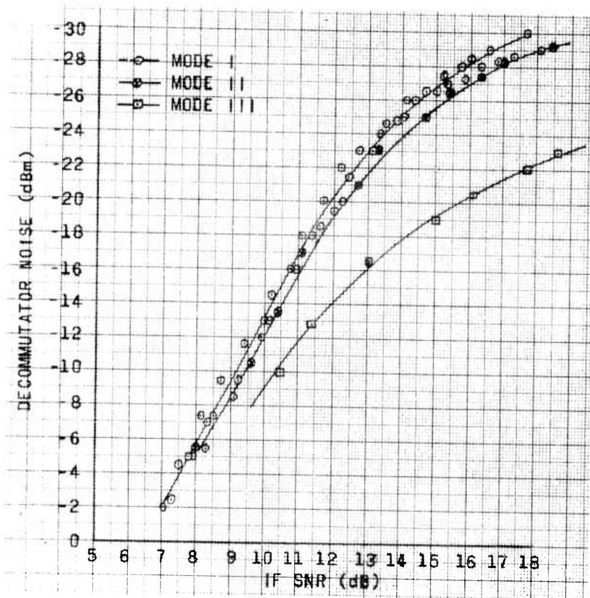
Figure 3. Relation Between Decommulator Noise and IF SNR.
