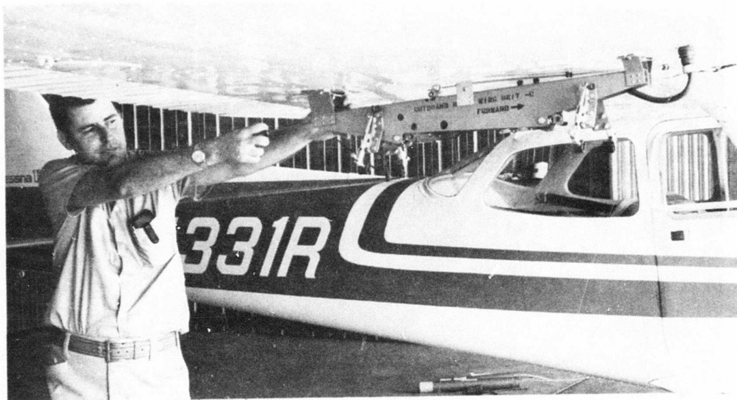
Figure 9. Shackle Cocking Procedure
