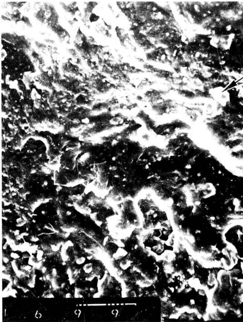
Figure 3.25 Suspected Area of Fracture Origin of Rotor Hub (1000 X)
