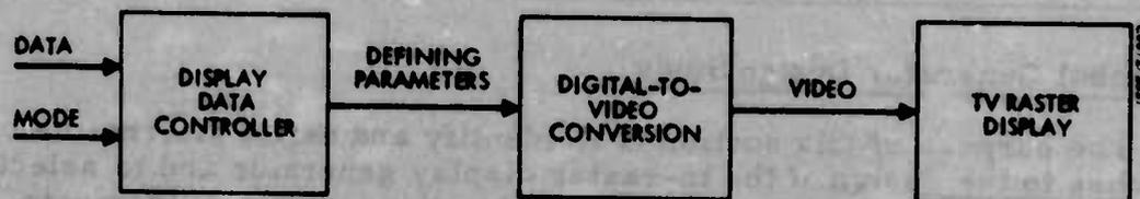
Figure 90. In-raster symbol generator/display system.
