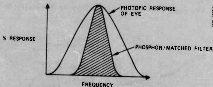
Figure 12. Narrowband phosphor/filter.
