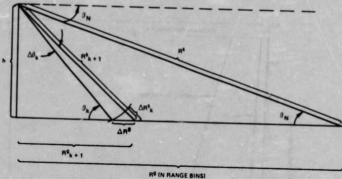
Figure 45. Ground range sweep correction geometry.
