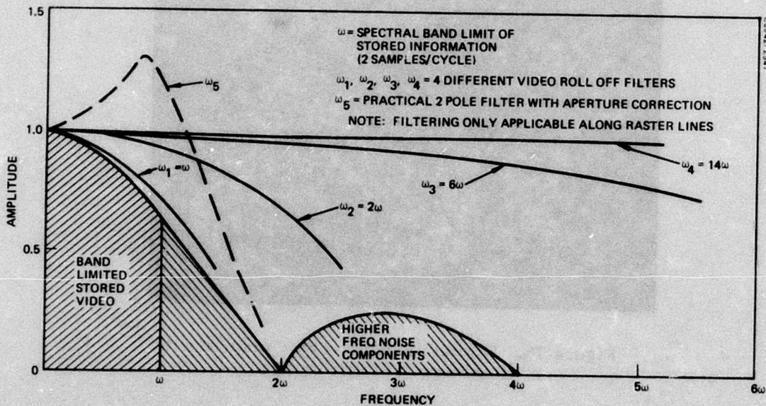
Figure 73. Bandpass characteristics of alternate video filters.
