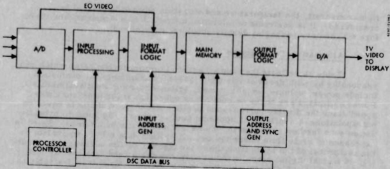
Figure 82. Final MMSDS digital scan converter architecture.
