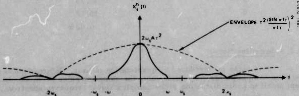
Figure 51. Sampled signal spectrum, long hold pulse.
