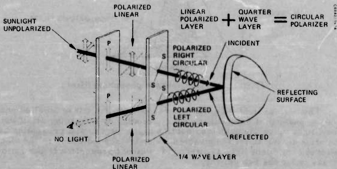
Figure 11. Circular polarizer.
