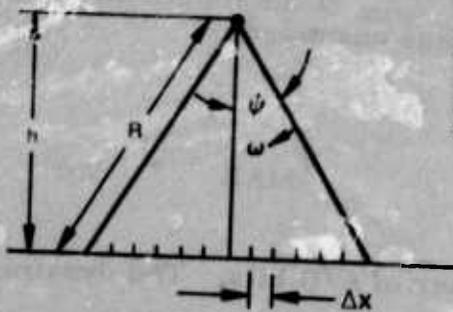
Figure 48. Geometry of downward looking line scan sensor.
