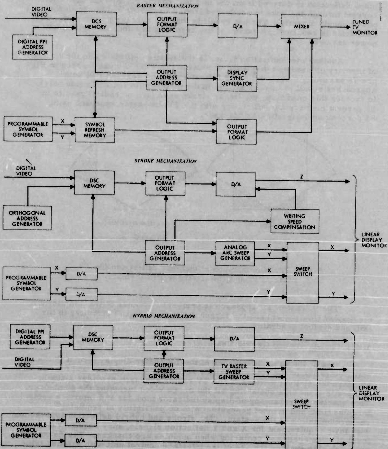
Figure 77. Alternate mechanizations.
