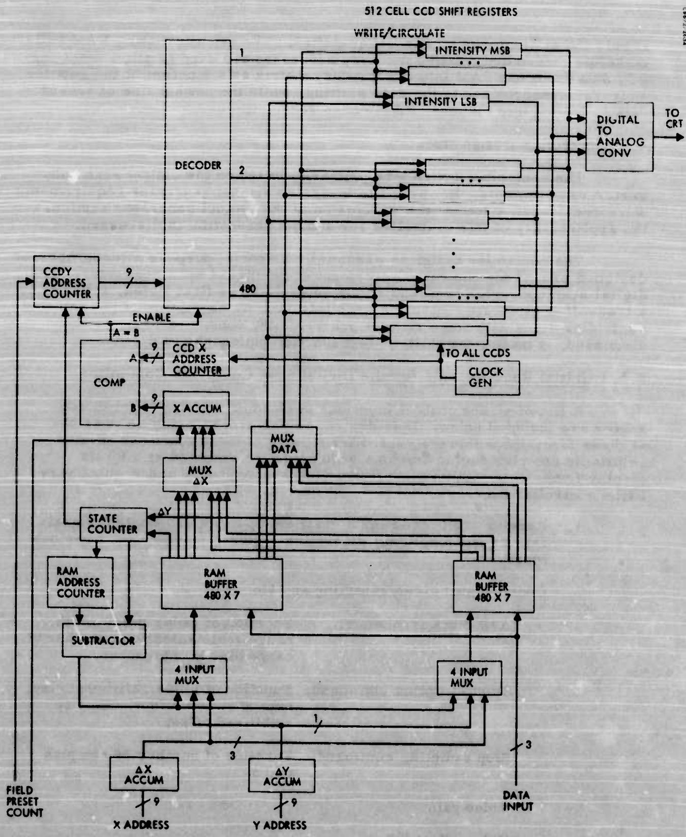
Figure 87. Display coordinate converter for a sequential access memory detailed block diagram.
