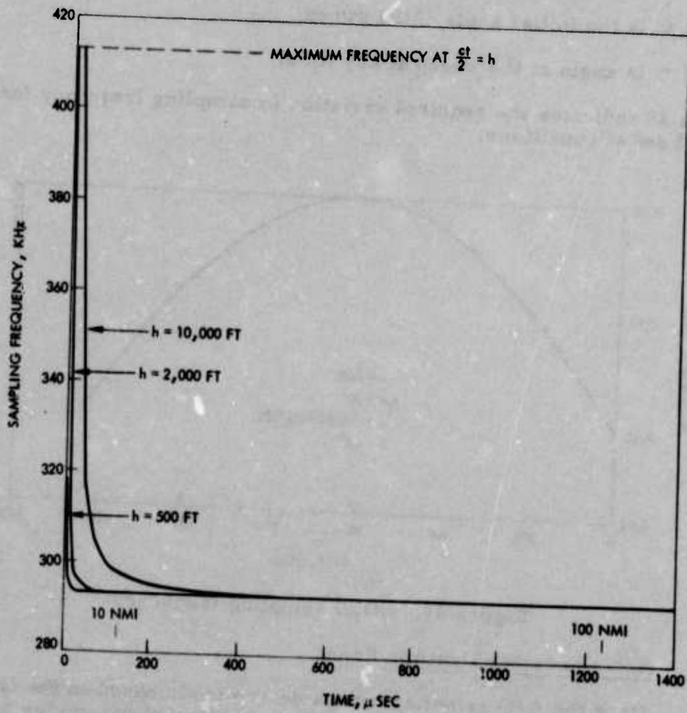
Figure 47. 100-mile ground range sampling requirement.
