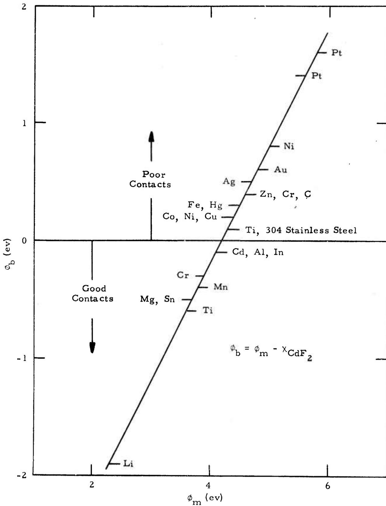
Figure 5. Estimation of Barrier Energies for Contacts on  $\text{CdF}_2$
