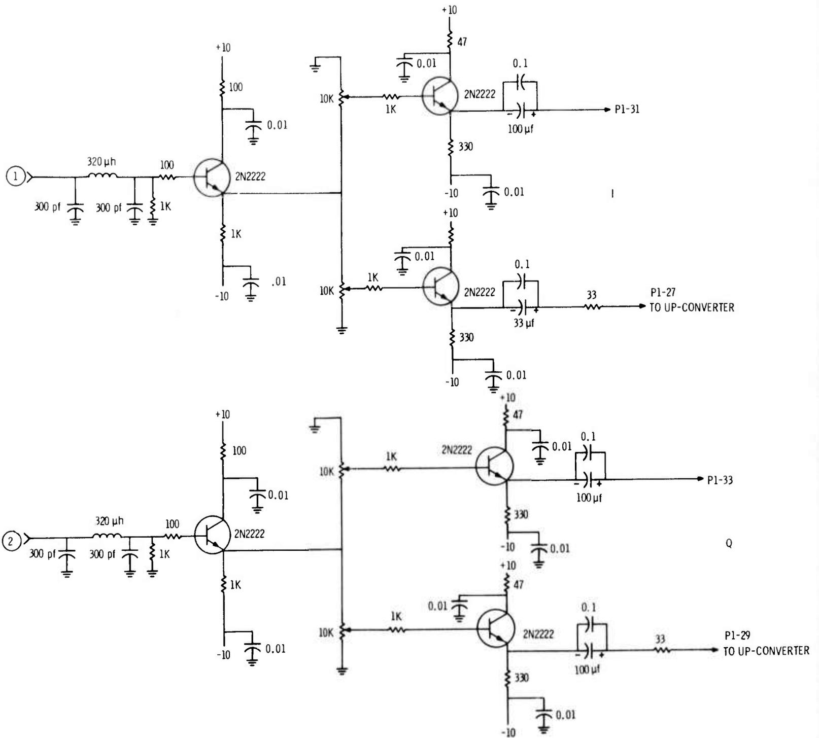
Figure 34. Input/Output Board - Output Section (Sheet 2 of 2)
