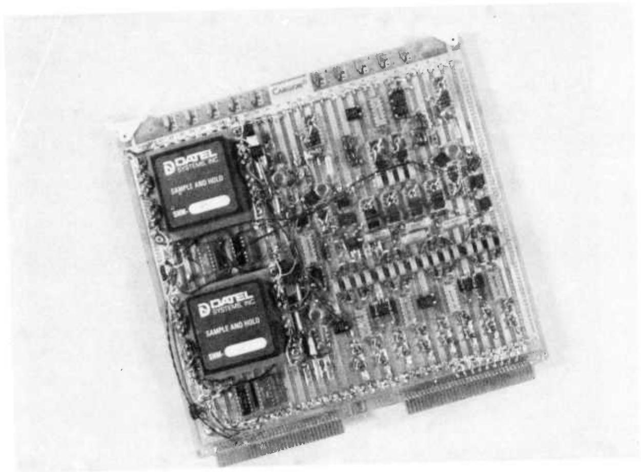
Figure 42. Input/Output Board
