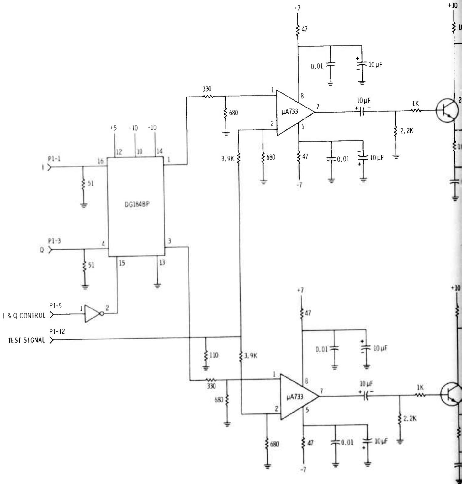
Figure 33. Input/Output Section
