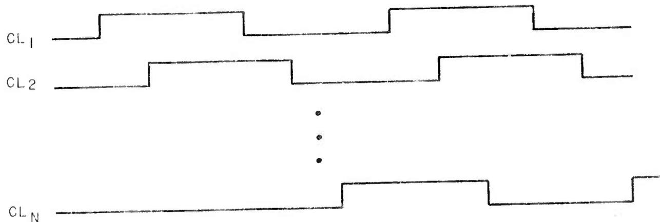
Figure 10. Overlapping Clock Operation
