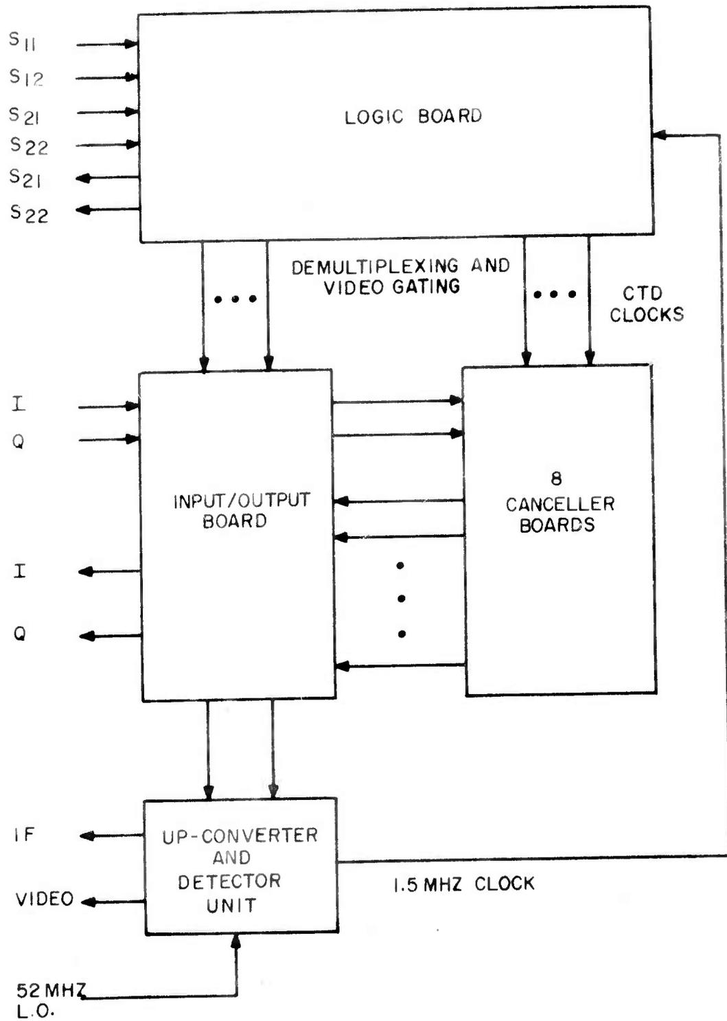
Figure 29. Discrete Signal MTI Block Diagram
