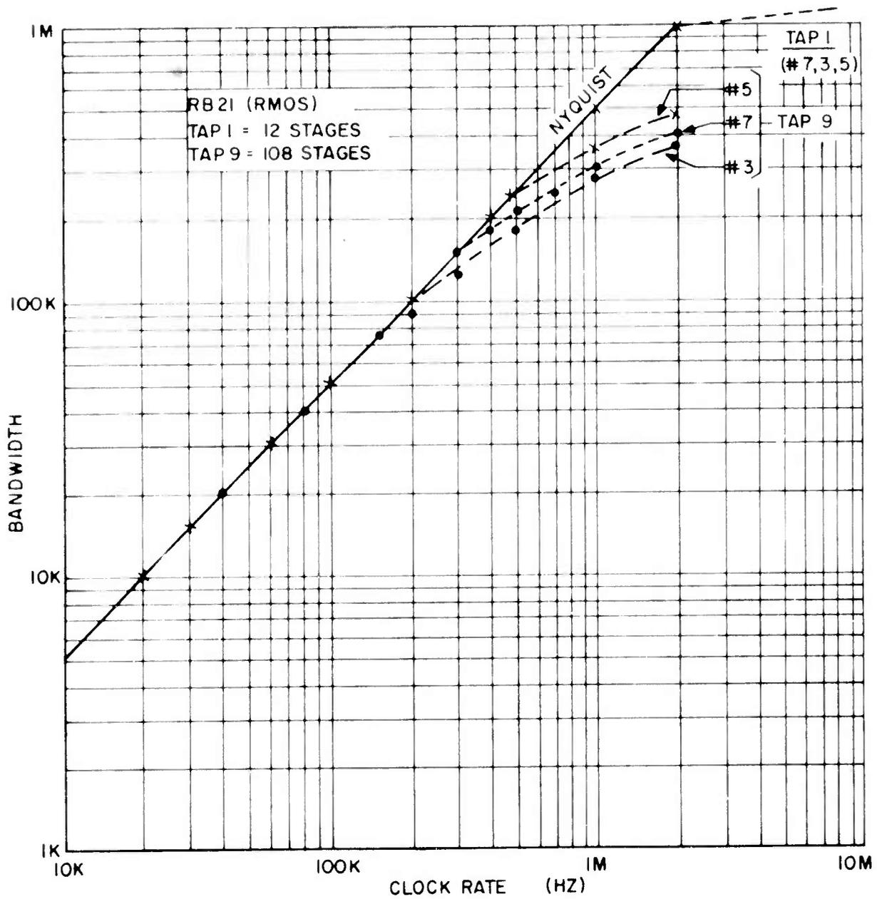
Figure 12. Clock Rate vs. Bandwidth for Typical Sample of Devices
