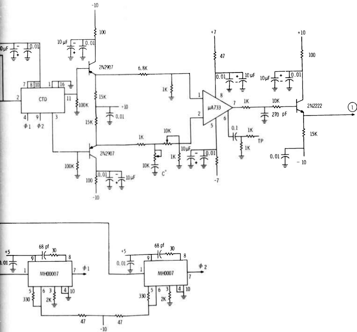
Figure 35. Cancellation Board - I Channel (Sheet 1 of 2)
