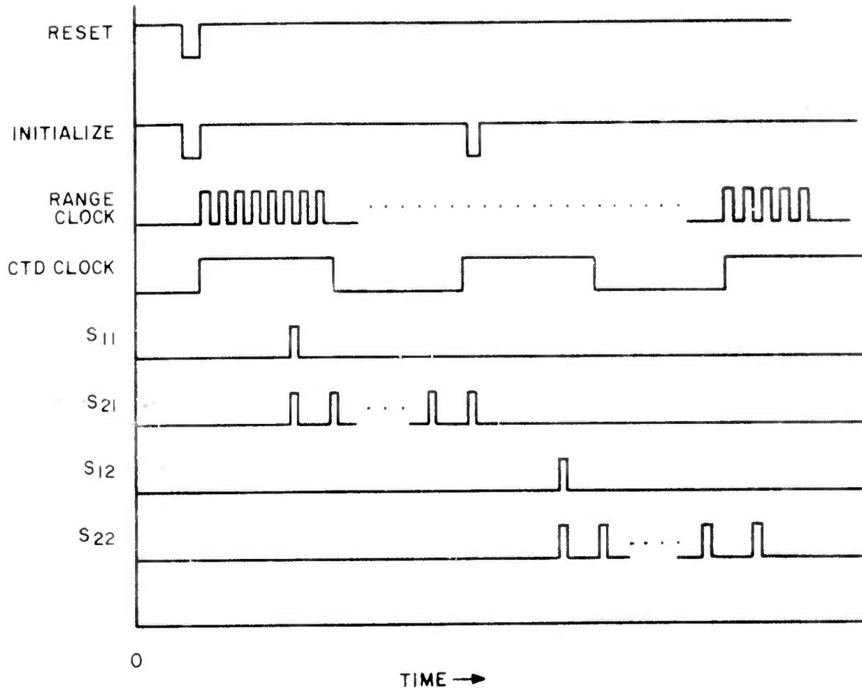
Figure 30. Logic Timing Diagram
