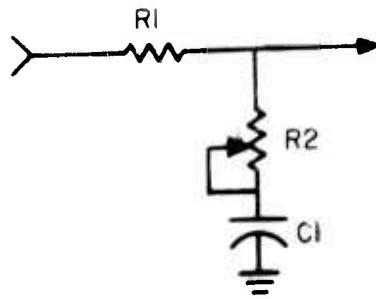
Figure 16. Compensation Filter
