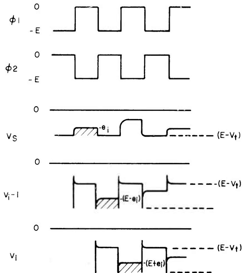
Figure 4. Nodal Voltage Waveforms for MOS CTD
