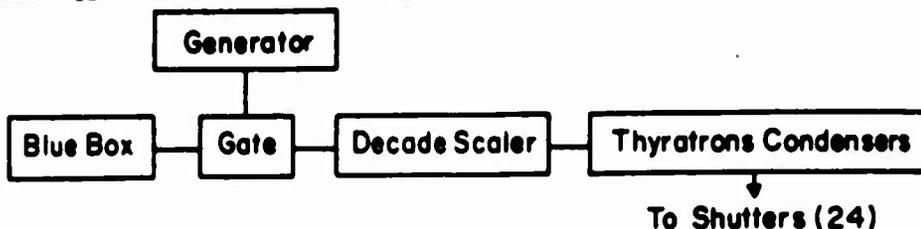
Figure 2.4 Box diagram for electronic timing of shutters.
