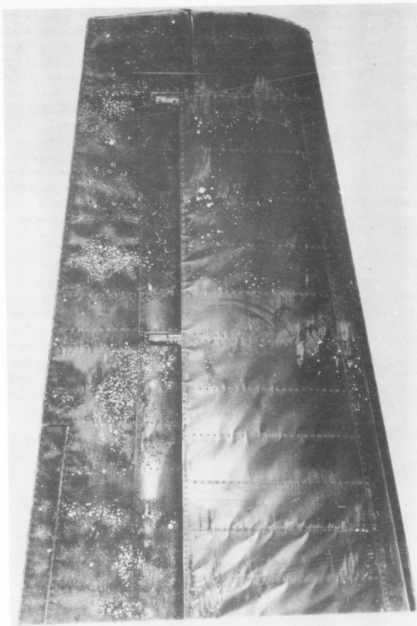
Fig. C.26 Over-all Damage Sustained by Stabilizer Exposed to Thermal Radiation Only, Station 3500, Shot 10
