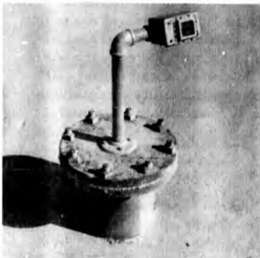
Fig. A.1 Typical Phototube Installation for Blue Box
