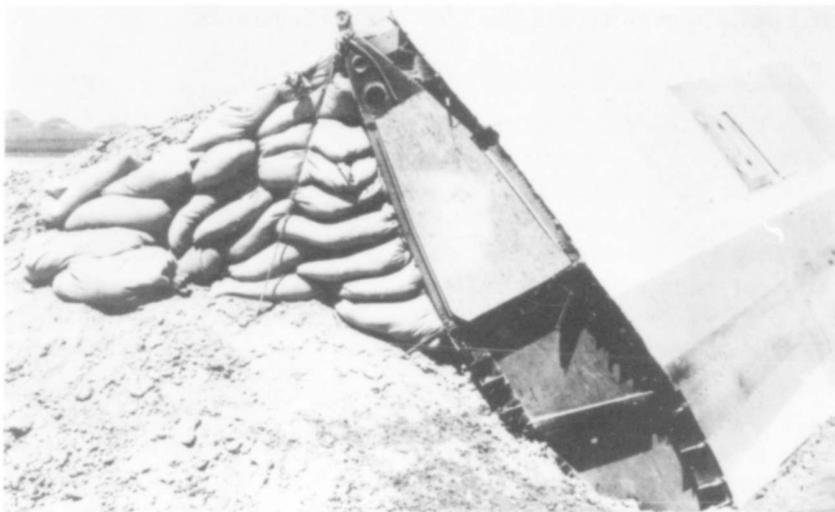
Fig. D. 44 B-36 Wing Section Prior to Shot 9, Range 4800 ft, Showing Plywood Bulkhead at Outboard Extremity
