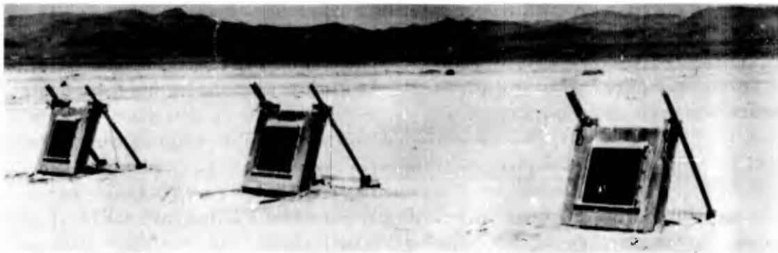
Fig. 2.5 Typical Bonded Metal Panel Blast Shield Array
