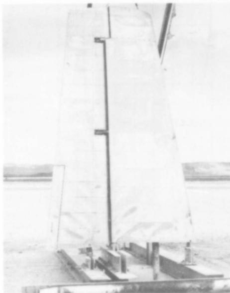
Fig. 3.4c Stabilizer Shielded From Thermal Station 6500, Shot 9
