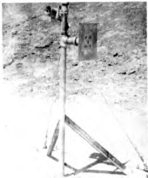
Fig. 2.10 Pressure Gage, Calorimeter and Mounting Assembly
