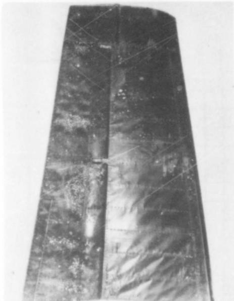
Fig. 3.3 Thermal Damage To Stabilizer at Range 3500, Shot 10
