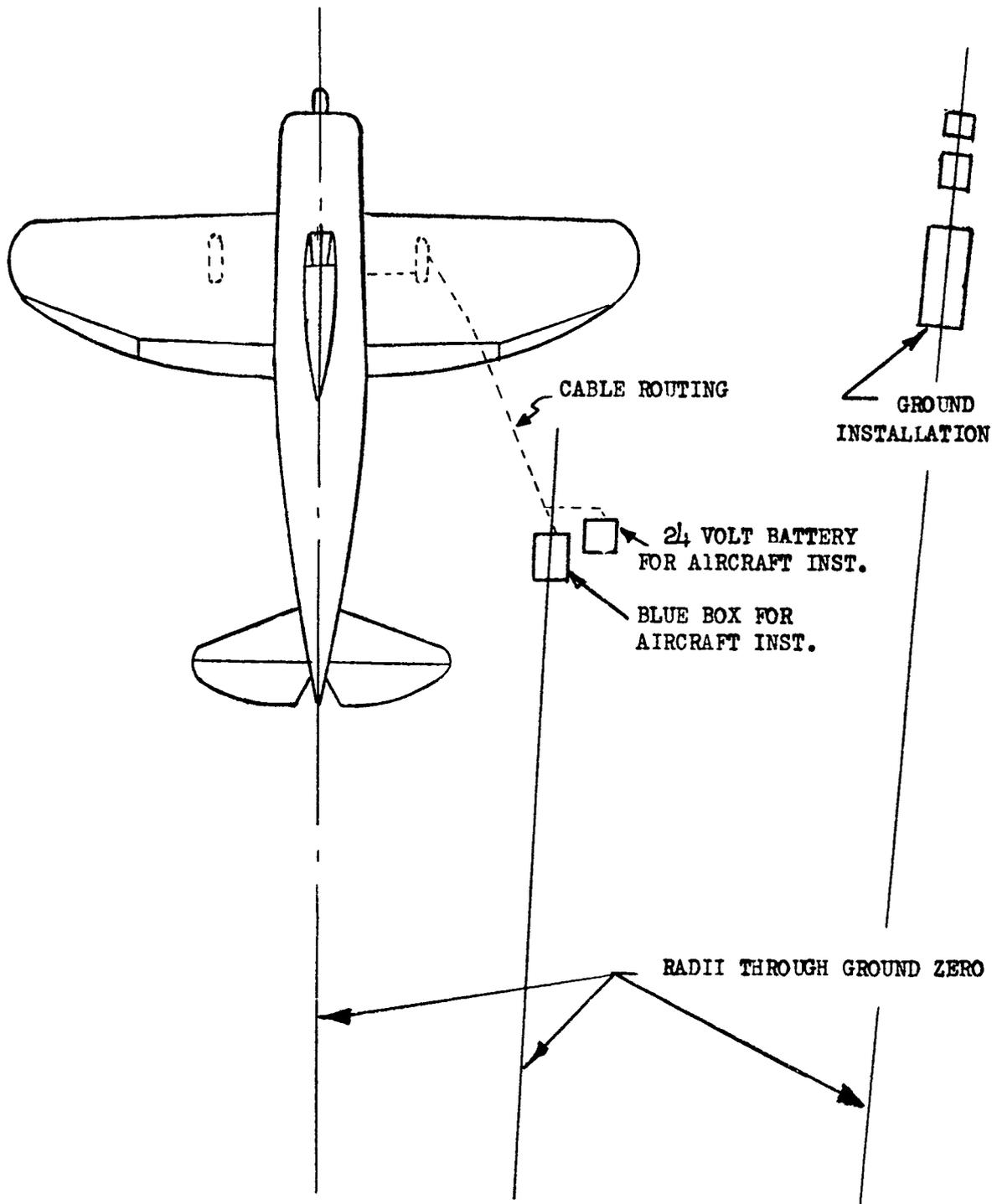
Fig. A.7 Schematic Diagram Showing General Location of Instruments
