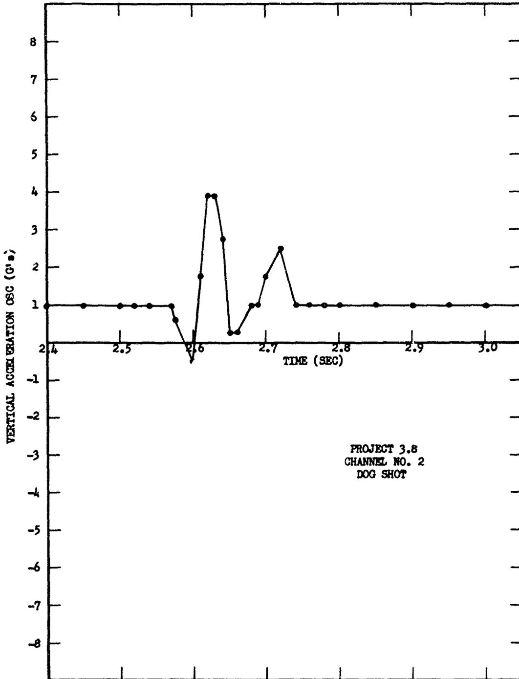
Fig. A.20 Ground Instrumentation Vertical Acceleration vs. Time
