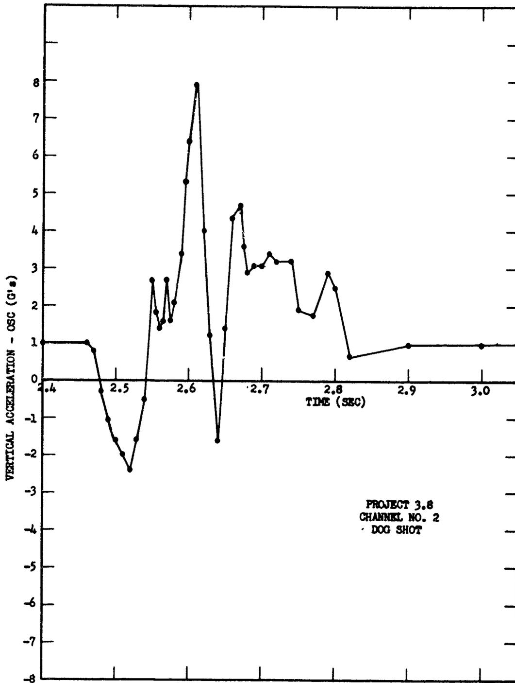
Fig. A.12 Aircraft Instrumentation Vertical Acceleration vs. Time
