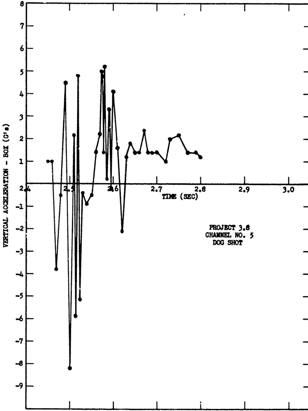
Fig. A.10 Aircraft Instrumentation Vertical Acceleration vs. Time
