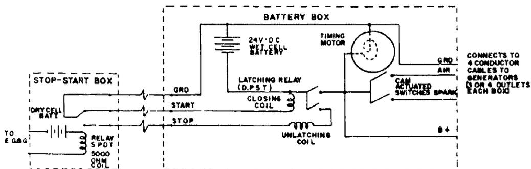
Fig. 2.16 - Circuit for Use with Smoke Generator, E19R3
