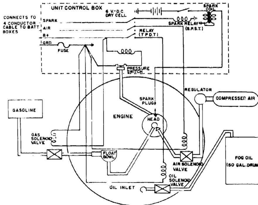
Fig. 2.15 - Control Arrangement for Smoke Generator, E19R3
