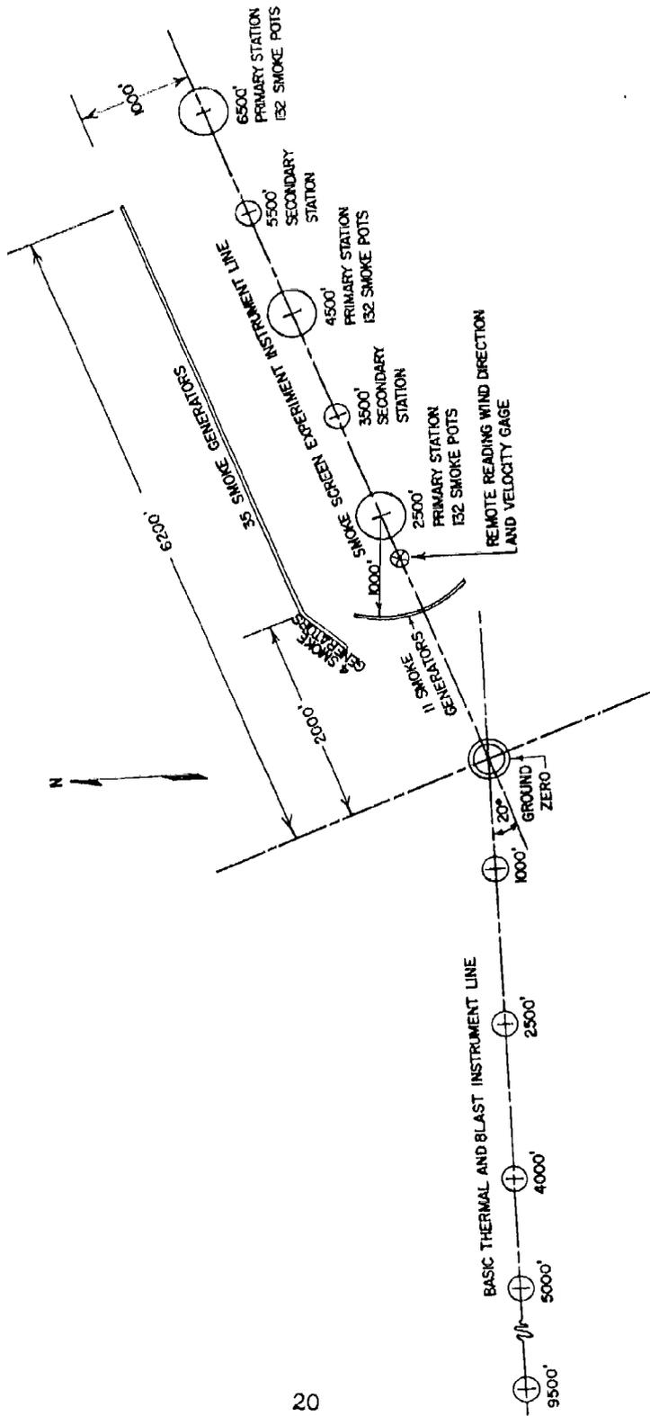
Fig. 2.1 Thermal Instrumentation Layout - Shot 9
