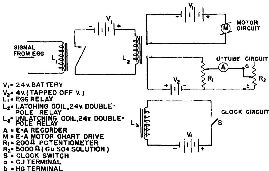
Fig. 2.12 - Circuit for Remote Control of Esterline-Angus Recorder
