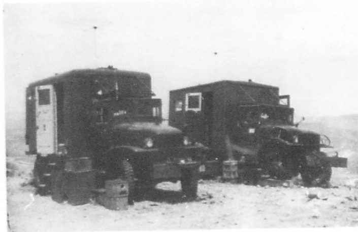
Fig. 2.4 Manned Stations. Note antennas for receiving signals from remote units.
