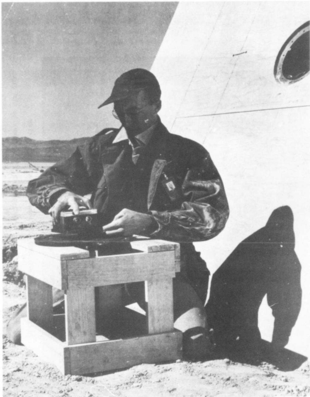
Figure 1.5 Attachment of Gage Head to Protective Drum Cover
