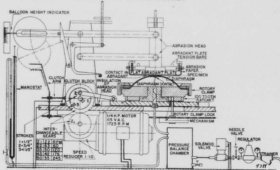
Fig. 2-DIAGRAM OF EDGE-ABRASION ATTACHMENT
