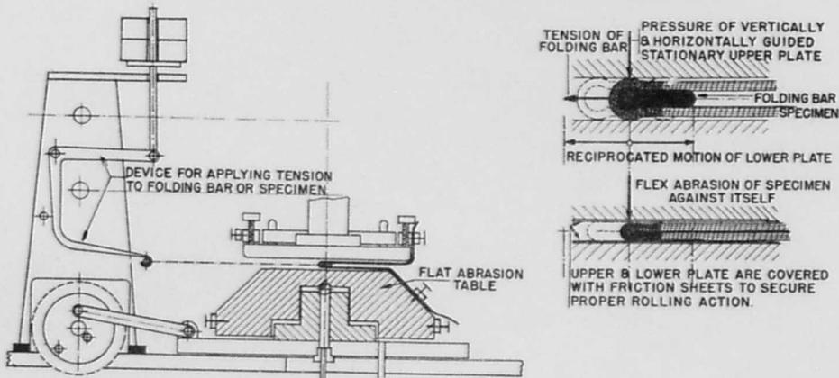
FIG. 4 - FRONT VIEW OF TESTER SHOWING FLAT ABRASED FABRIC IN PNEUMATICALLY CONTROLLED ROTARY SAMPLE CLAMP
