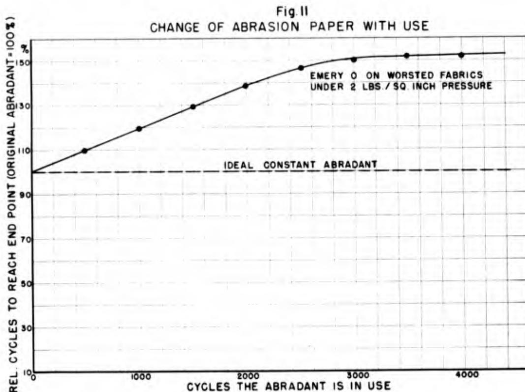
For flat- and edge-abrasion testing with this instrument the abrasion papers Emery O and water-resistant silicon carbide No. 600 have shown satisfactory qualities and can be recommended. The construction of the flat-abrasion plate makes it possible to use a single abrasion sheet for several tests by slightly shifting the abrasion area after each test.
