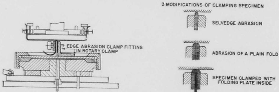
Fig. 3 - DIAGRAM OF FLEX ABRASION ATTACHMENT
