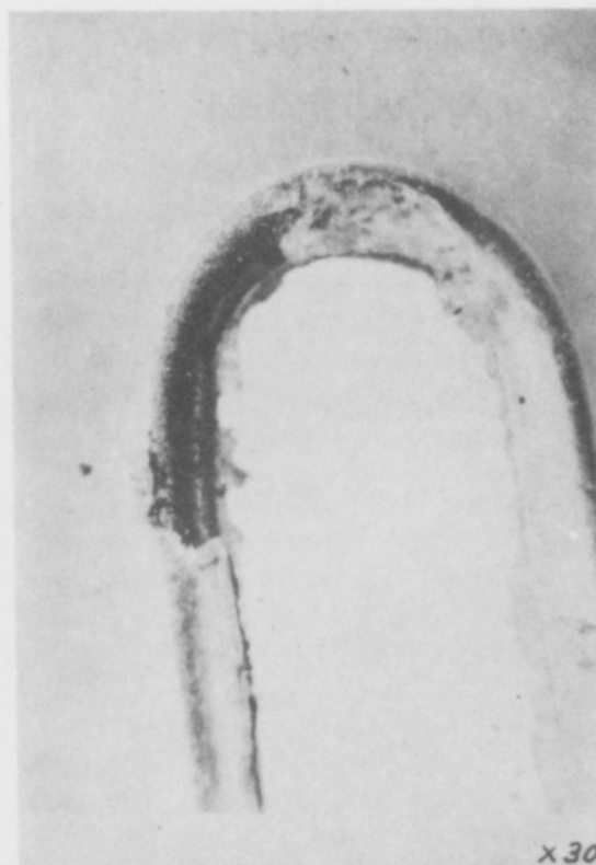
PLASTIC HEDDLE x10 Showing Cracked Plastic Over Metal
