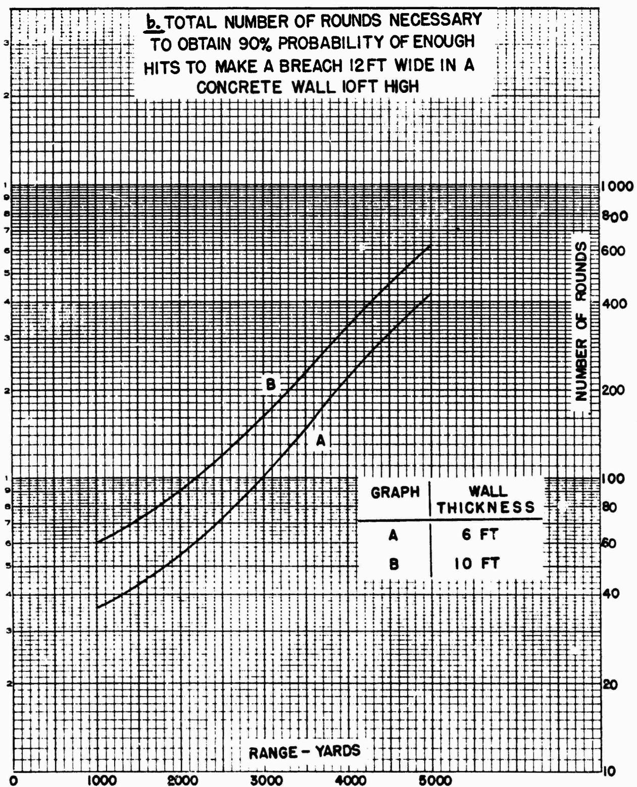
**11. Effectiveness.** The following data on effectiveness of HE Shell M107 with PD Fuze M51A4 or MT Fuze M87A3, fired from the 155-mm Howitzer M1, were taken from volume III of "Terminal Ballistic Data".
