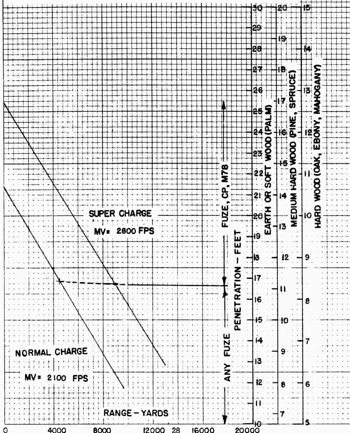
b. PENETRATION INTO MEDIUM EARTH AND LOGS.
