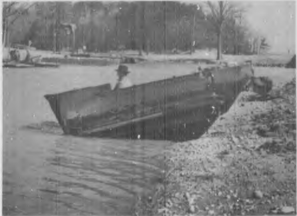
FIGURE K. The M29C Cargo Carrier entering the water with rudders and splash shield in position.
