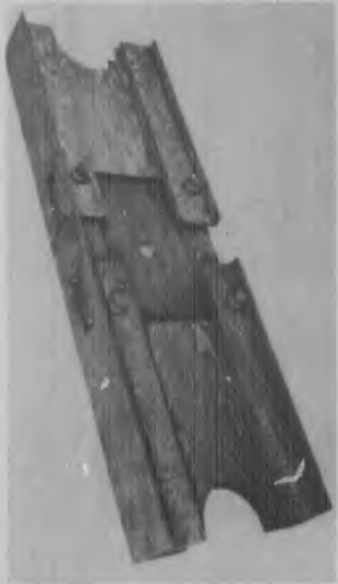
Connector assembled as a moment joint.
