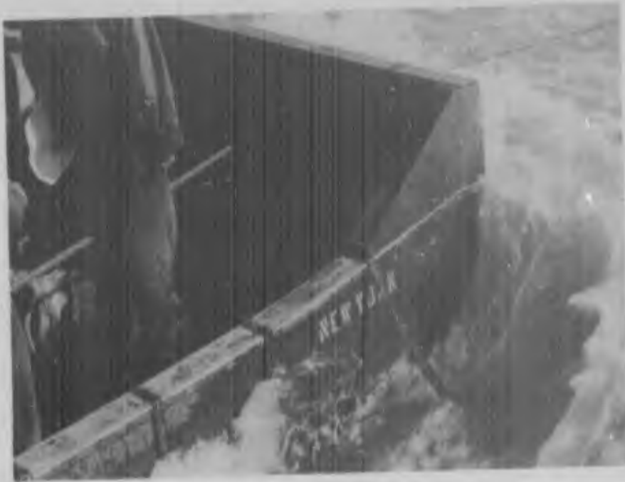
Adapter to increase height of bow to prevent swamping.
