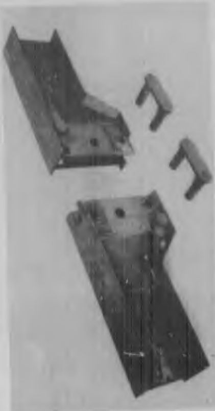
Locking pins and shear lugs are removed and links are turned into balk ends by operating link handles. Balk are now free to be separated in any direction.
