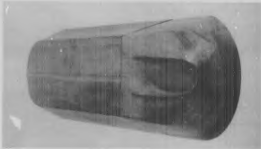
FIG. 55. STERN VIEW OF POWER ADAPTER. Stern views of two types of power adapters studied in model tests. The adapter to the left was found more effective and the pilot model is being constructed in accordance with this model.
