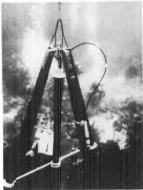
A typical magnetometer array structure being inspected by divers.
