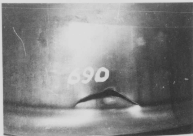
Helmet S1. Schlueter 213B7. -C- Edge Annealed. Impact 1.2" up from rim at 255°.
