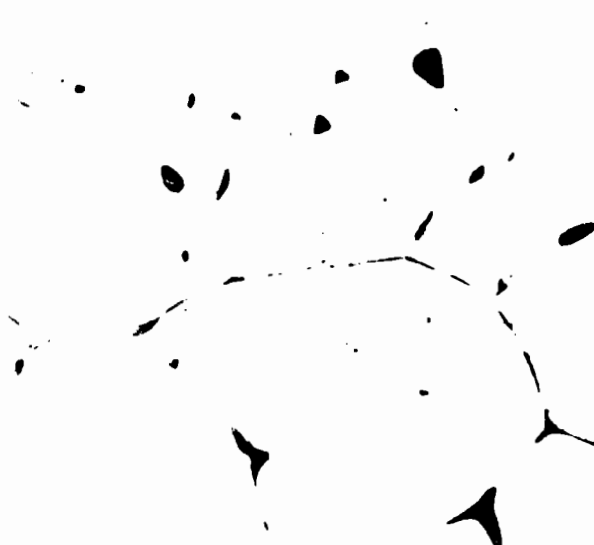
X100 Unetched Occasional segregated area of sul- phide inclusions in the primary grain boundaries.
