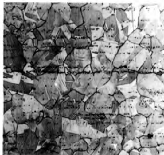
Helmet No. 95 McCord Lot No. 165 Streaks of globular carbides and grain boundary carbide network.
