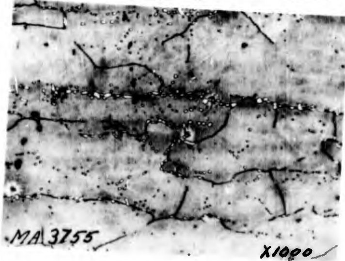
FIGURE 3 TYPICAL STRUCTURE OF POOR FORMING STEEL LOT * C.I. 254463 MC C. 28C
