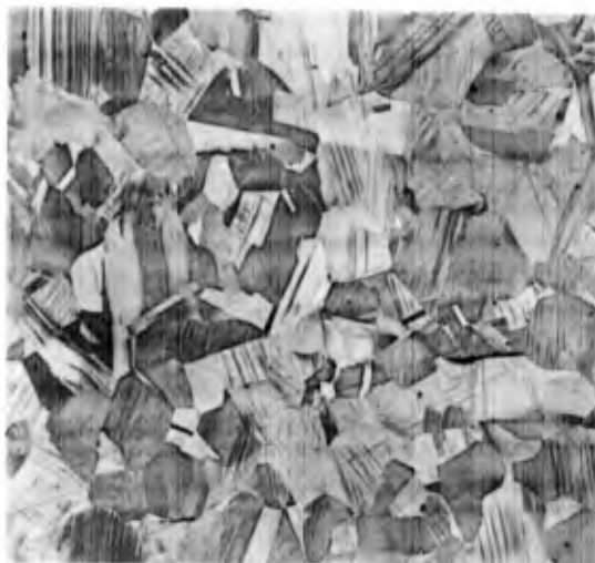
Helmet No. 93 McCord Lot No. 149C Satisfactory microstructure. No undissolved carbides.
