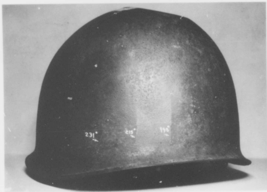
Helmet No. 79. McCord Lot 40B1. Camp Pickett. Mag. X \frac{1}{2} Body cracks at back of helmet. Numbers refer to positions shown in Figure 1.
