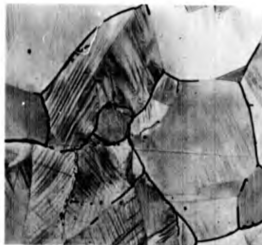
Helmet No. 92 McCord Lot 148B Grain boundary carbide network.
