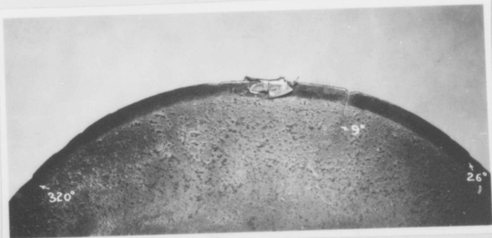
Helmet No. 98. McCord Lot 149A. Camp Livingston. Mag. XI Edge cracks at visor of helmet. Crack at 9° definitely associated with notch. Stainless steel edging has been removed.
