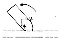
G. THE INITIAL REACTION FORCE EXERTS A COUPLE WHICH TURNS THE PRO-JECTILE SO AS TO LIE PARALLEL TO PLATE.
