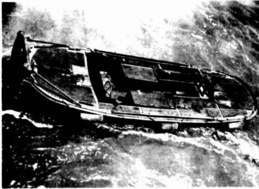
FIG. 17. DECK ARRANGEMENT OF TWIN-SCREW UTILITY POWER BOAT, T-3. Showing arrangement of cockpit, control station, equipment and large forward working deck.
