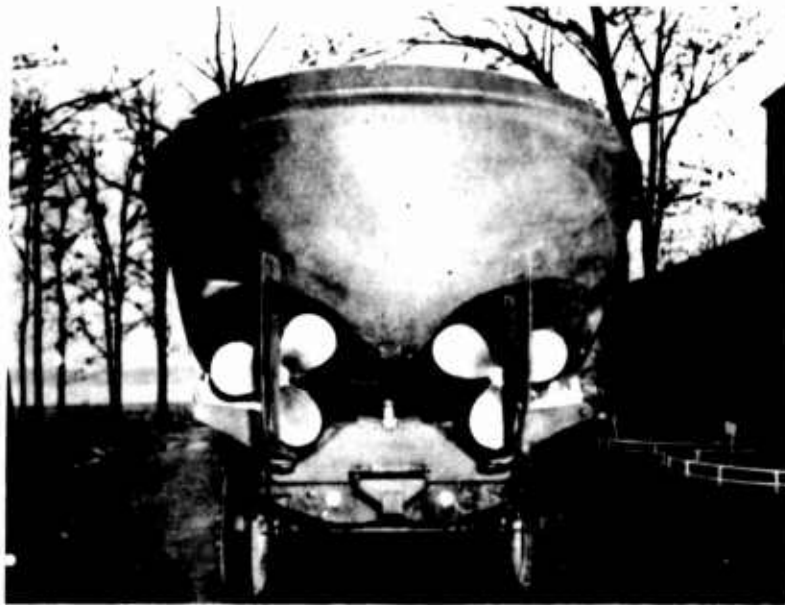
FIG. 22. STERN VIEW OF TWIN-SCREW UTILITY POWER BOAT, T-3, ON POLE-TYPE TRAILER. Note extent of tunnels and location of 26-inch diameter propellers in tunnels, which assist greatly in maintaining a minimum draft of 32 inches.
