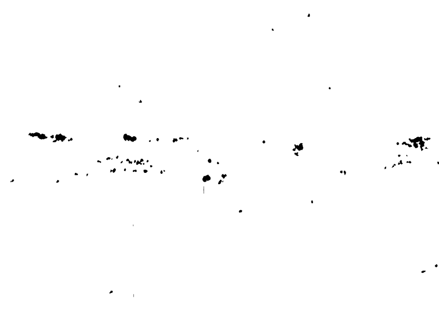
X100 Light Micro Etch Plate #2 - A segregation of friable alumina type nonmetallics occasionally found in laminated areas.
