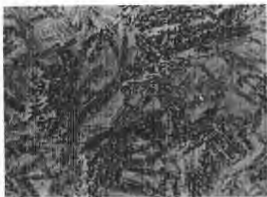
K Heat 9 L Martensite and resolvable bainite. Rc 49. Martensite, resolvable bainite and ferrite. Rc 42.
