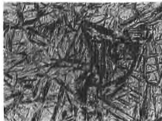
Heat 16 X Martensite and a small amount of acicular bainite. Rc 50.
