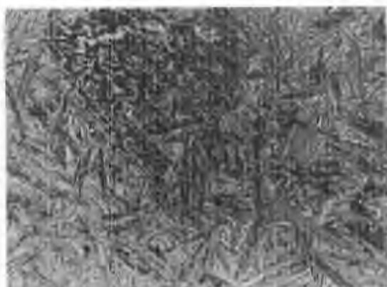
I Heat 8 J Martensite and resolvable bainite. Rc 47. Bainite and a small amount of ferrite. Rc 40.
