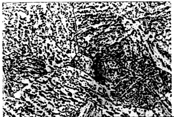
X1000 Nital Picral Outer third of cross-section. Sorbite and grain boundary carbides. Very little free ferrite.
