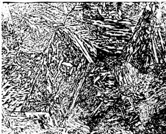
X200 Nital Picral Middle of cross-section. Large amount of free ferrite.
