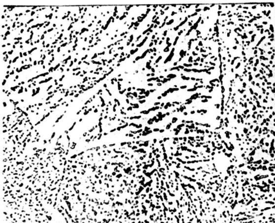
X1000 Nital Picral Middle of cross-section. Carbides, ferrite, and grain boundary carbides.
