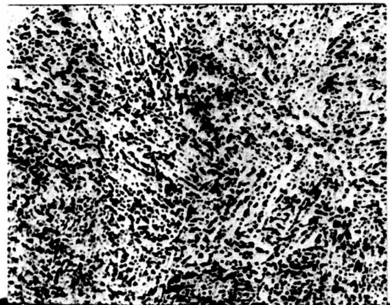
X1000 Nital Picral Outer third of cross-section. Uniformly spheroidized sorbite. No free ferrite.
