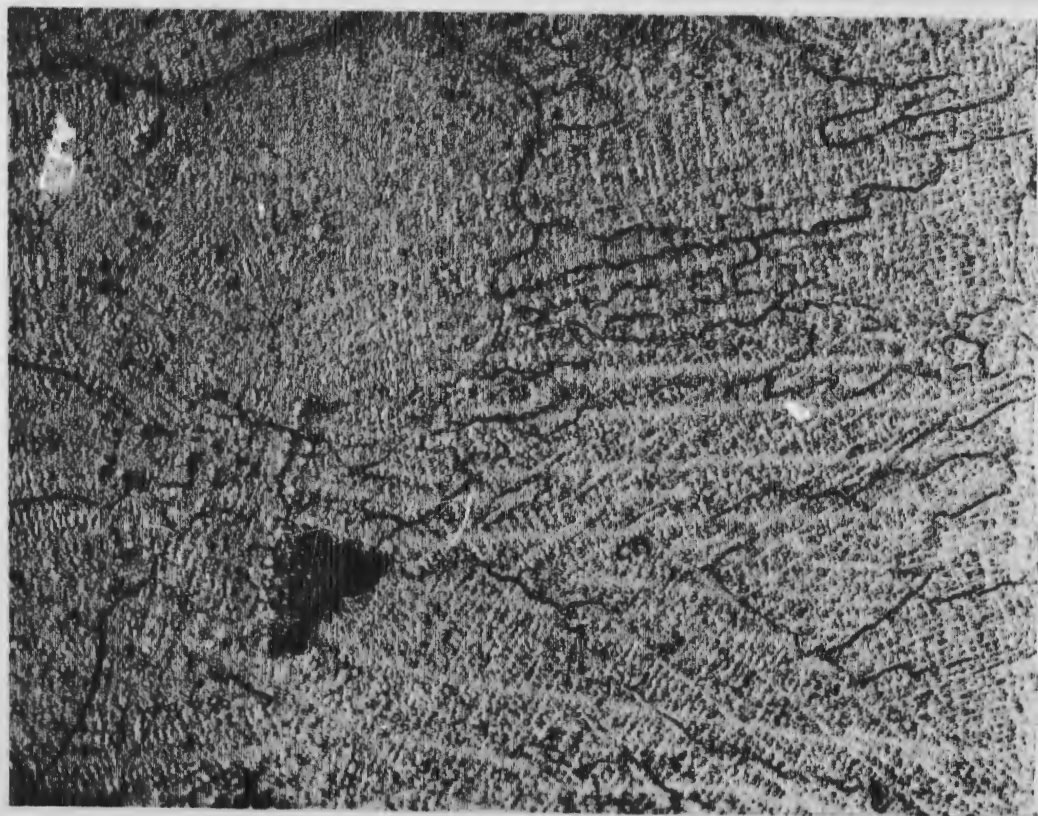
Hot Acid Etch. Lower right hand corner of above photo. X5 Heavy etching attack at dendrite boundaries.
