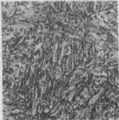
#E X200 As received. Coarse, segregated structure.
