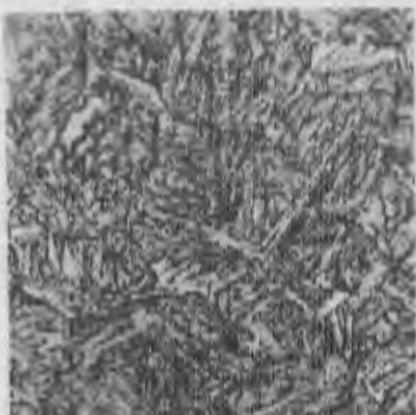
#H X1000 Reheat-treated. Small amount of rejected ferrite and pearlite in tempered martensite.
