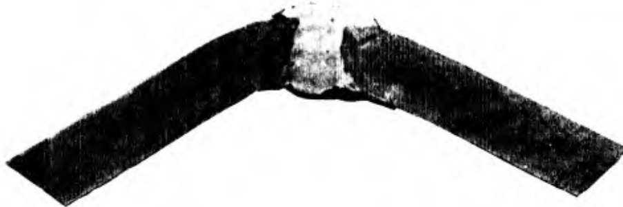
1/2 inch thick austenitic hand welded rolled plate General Motors Truck C 11 - tested at room temperature
