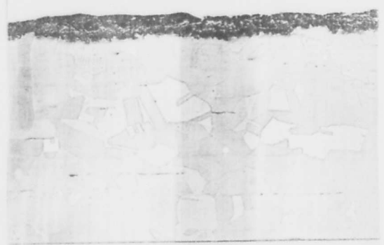
B Disc No. 12 X100 Light Nital Oxide layer on surface of steel not high magnetic. No martensite layer.
