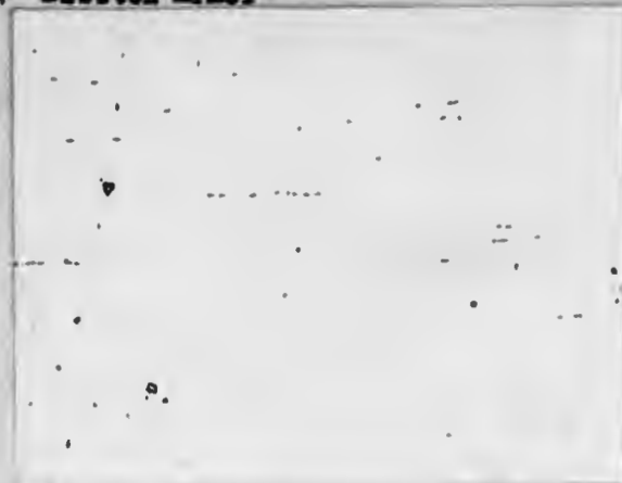
X100 B Unetched Plate #3 - typical distribution of inclusions.
